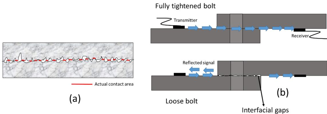
Figure 6: (a) Microscopic gaps at the plates interface (b) wave propagation in fully tightened loosely bolted specimen
