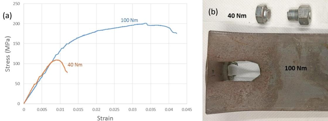
Figure 1: (a) Stress-strain behaviour of bolted joint at 100 Nm and 40 Nm (b) failure of specimens at 40 Nm and 100 Nm bolt torque (Jay Kumar Shah 2019)
