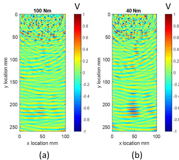
Figure 5: Images of bolted plates at (a) 100 Nm and (b) 40 Nm bolt tightening
