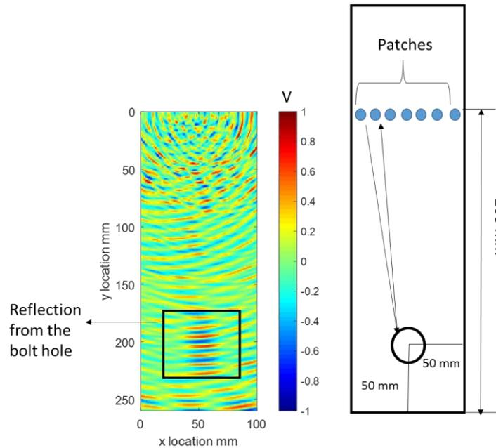
Figure 4: Developed image of a single plate with bolt hole
