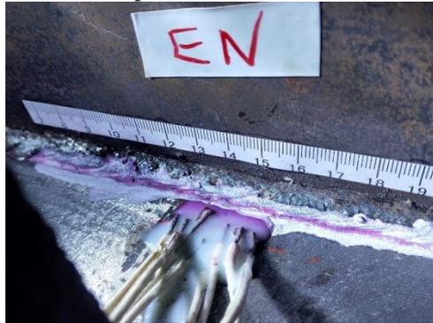
Figure 4: Typical fatigue cracks at stiffener-to-web weld toes.
