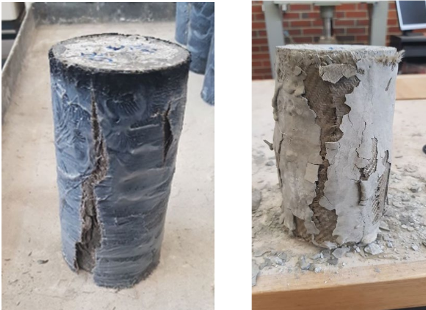
Figure 4. Failure of BFRP confined specimens bonded by epoxy (left) and geopolymer (right).
