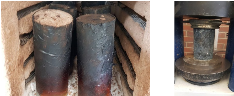
Figure 3. Heating of the specimens in a furnace (left) and compression test after cooling (right)
