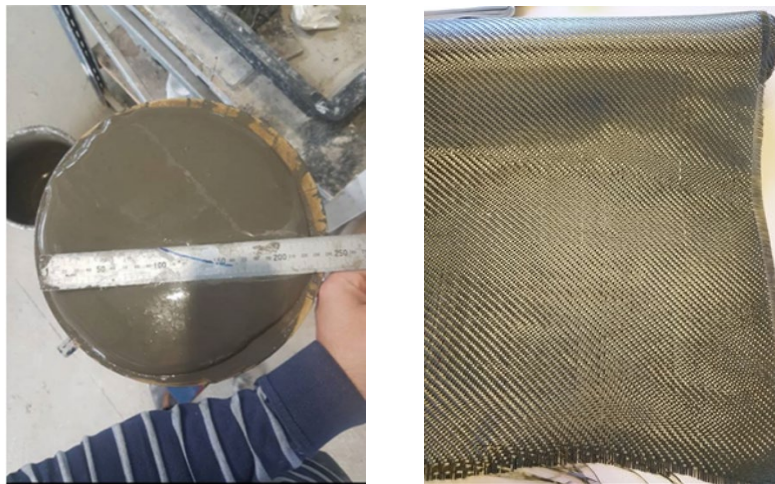
Figure 1. Geopolymer paste (left) and BFRP fabric (right).
