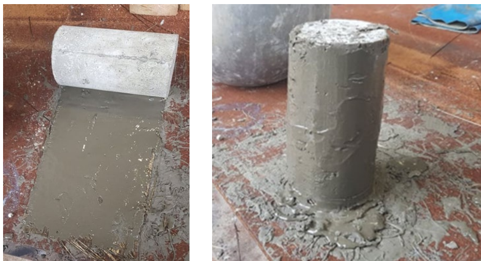
Figure 2. Wrapping of BFRP fabric to concrete cylinders by geopolymer paste.
