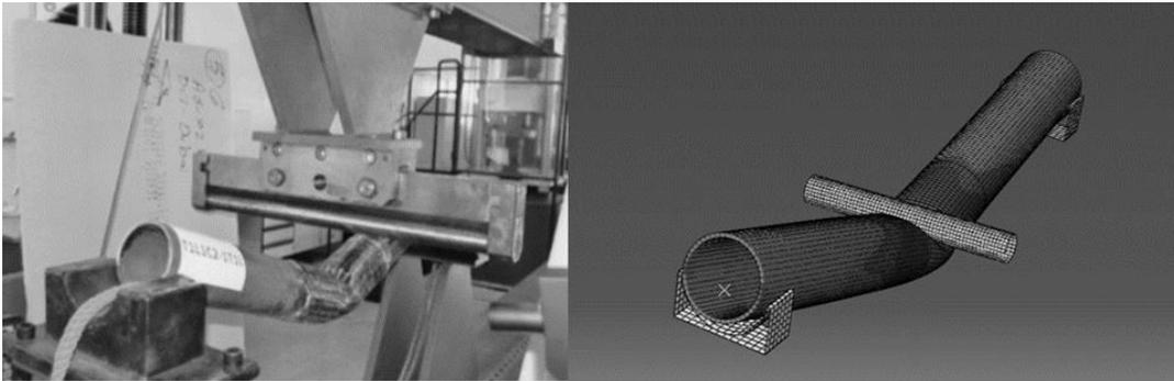
Figure 2. Comparison of the experimental specimen [left] with the FE model [right].
