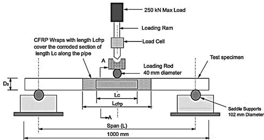
Figure 1. Experimental set up for three-point bending, Elchalakani (2016).
