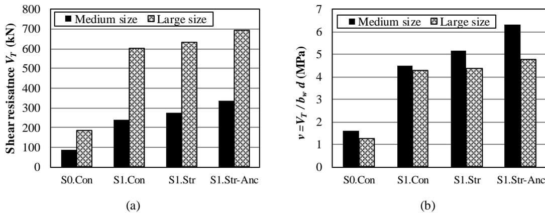
Figure 3. Shear behavior with increasing beam's size: (a) Shear resistance and (b) Shear strength.
