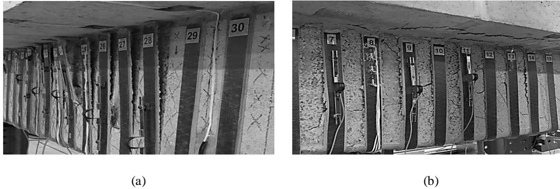
Figure 2. Shear failure: (a) CFRP laminate debonding in L.S1.Str; and (b) CFRP laminate debonding in L.S1.Str-Anc without anchorage pullout.
