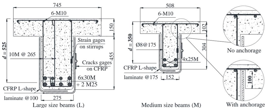
Figure 1. Cross section of specimen's and strengthening system (dimensions in mm).
