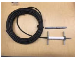
Figure 1. Typical H-gauge used in APT test facilities in the United States.
