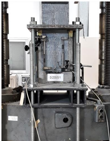
Figure 3. Single shear test set up.
