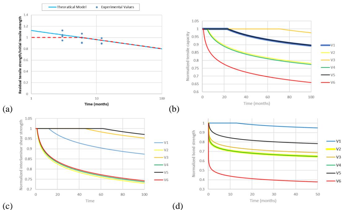
Figure 3. Predicted evolutions of mechanical performances (a) Example of model correction due to post curing (for tensile strength under V4 conditions) (b) Tensile strength (c) Interlaminar shear strength (d) Bond strength
