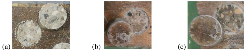
Figure 2. Failure modes (a) Cohesive concrete failure (b) Mixed failure- debonding and cohesive concrete failure (c) Debonding of the laminate
