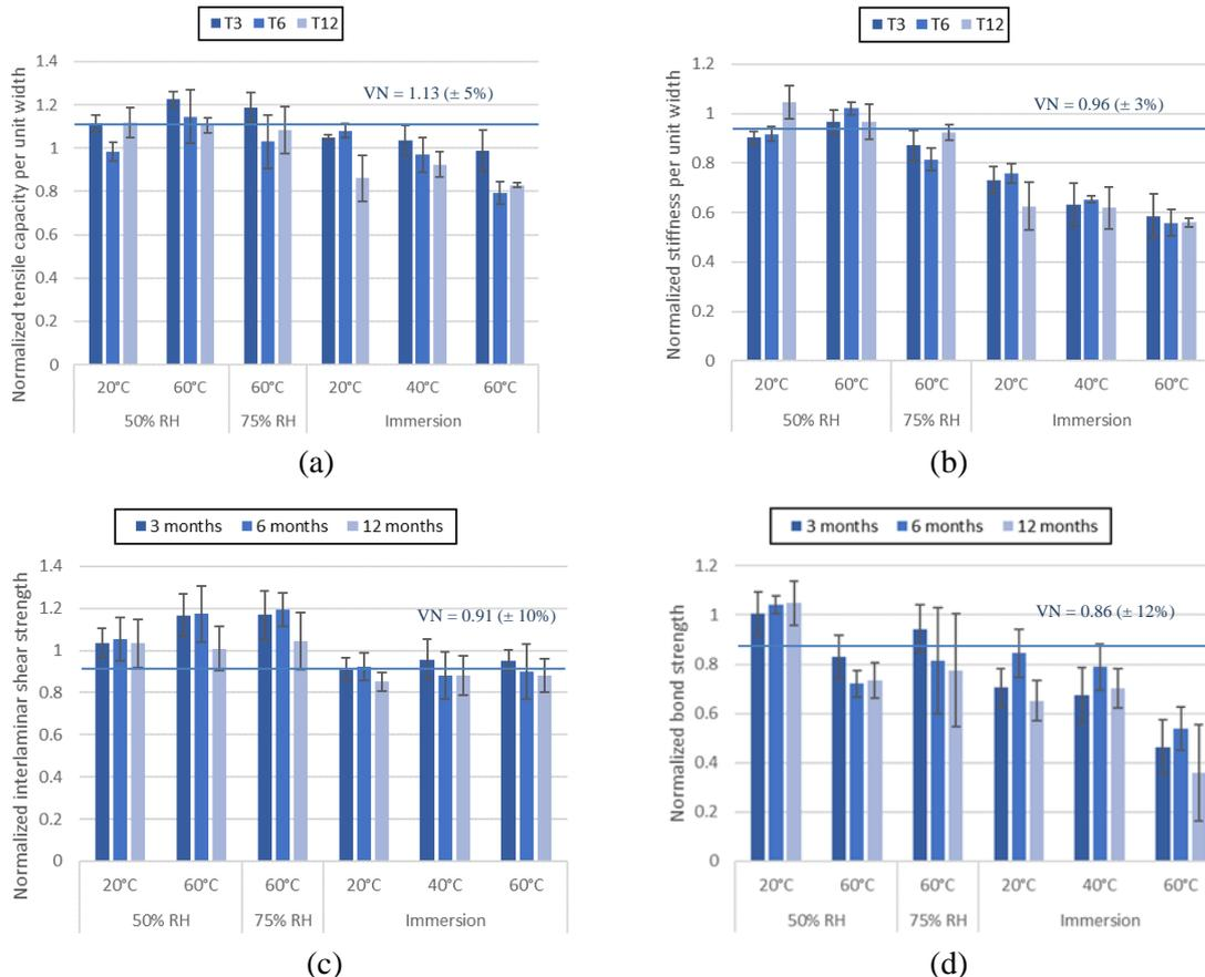
Figure 1. Normalized results of mechanical tests (a) Maximum tensile force per width unit (b) Tensile stiffness per width unit (c) Interlaminar shear strength (d) Pull-off bond strength, for specimens exposed up to 12 months.
