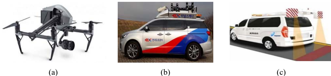
Figure 3. Imaging equipment used for crack detection: (a) DJI inspire 2 drone, (b) tunnel imaging car and (c) road scanning car
