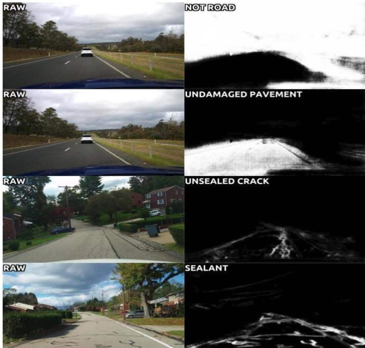
Figure 2. Selected segmentations from our deep learning model. Left column contains raw video frames. Right column contains model output where grayscale value indicates probability (i.e. black = 0%; white=100%).
