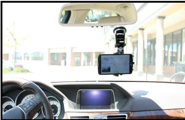
Figure 4. An android phone running custom software records video, GPS, and accelerometer data. A second phone is used for turn-by-turn navigation (not shown).
