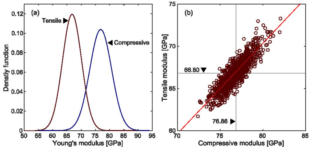
Figure 2. Gaussian copula. (a) Marginal density functions of the tensile and compressive moduli; (b) bivariate sample of 1000 points of a Gaussian copula.
