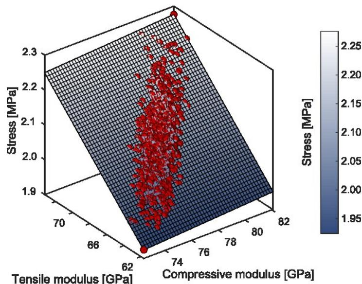
Figure 4. Response surface of the maximum tensile stress. Note: The red circles represent data obtained for the stochastic case.
