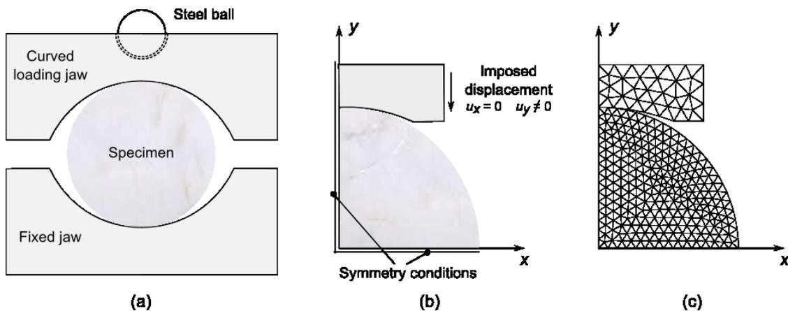
Figure 1. Brazilian test setup. (a) Test specimen; (b) simplified model; (c) finite element mesh.
