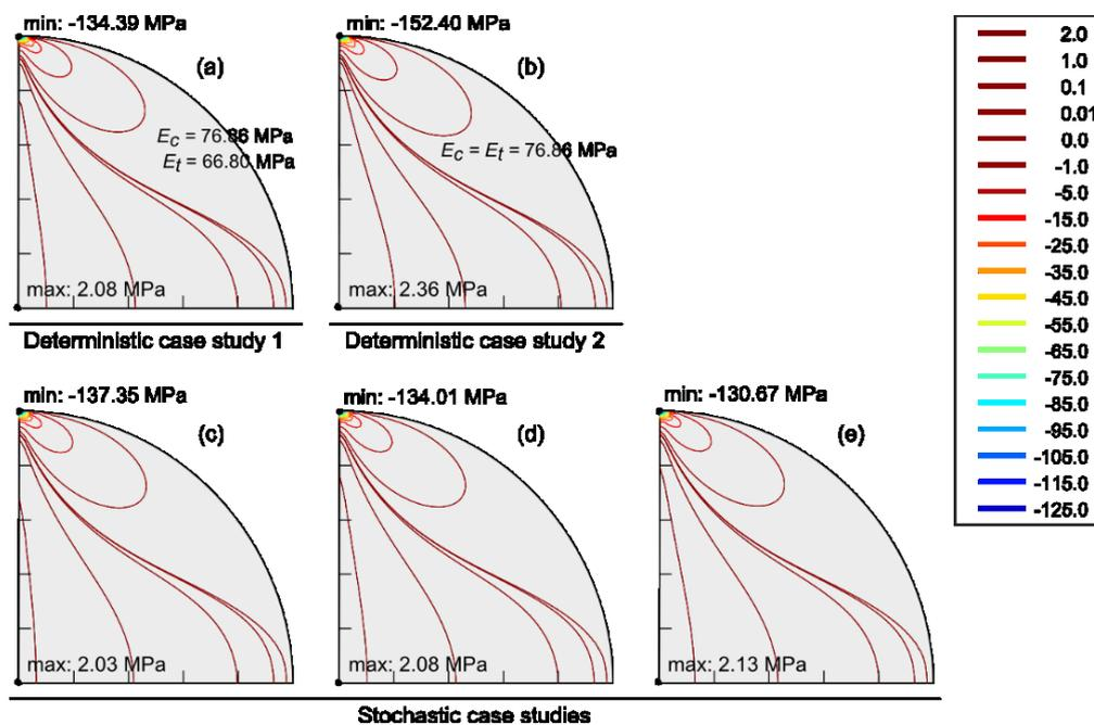
Figure 3. Stress distribution along the x axis of study cases. Normal stress values are expressed in MPa.
