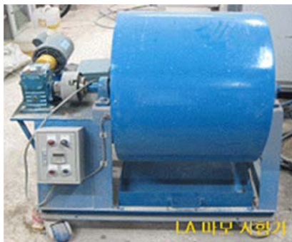
(a) Los Angeles Abrasion Test
