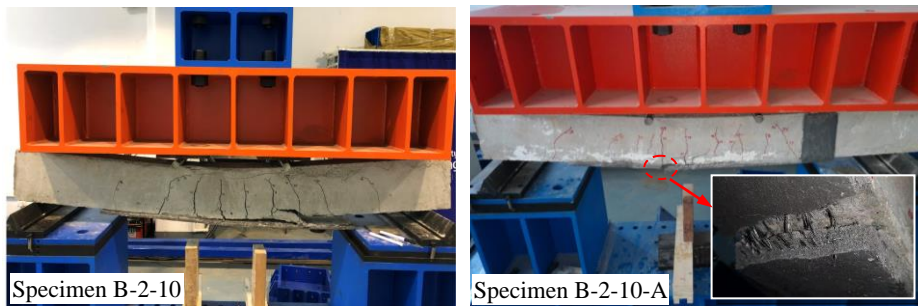
Figure 5. Failure modes of strengthened beams.
