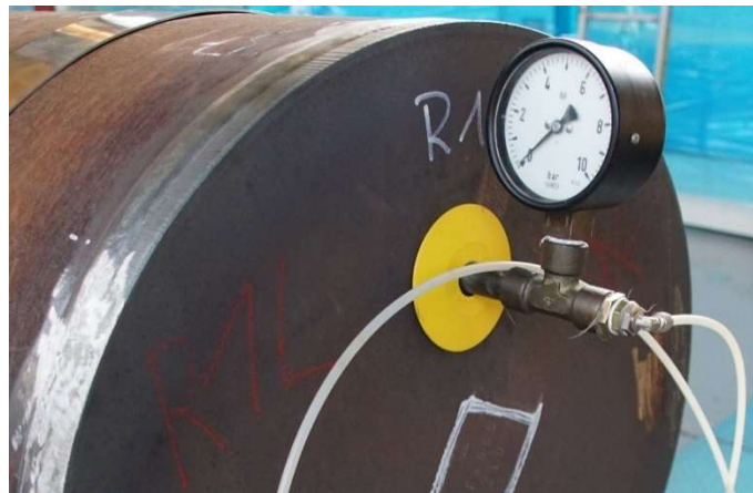
Figure 2: Measurement of inner pressure with analog and digital devices on tube
