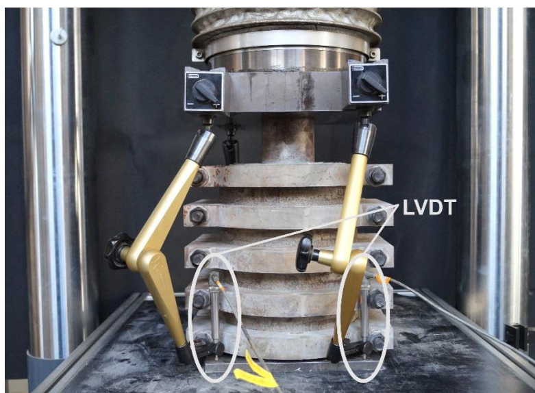
Figure 3. Specimen placed in the servo-hydraulic testing machine.
