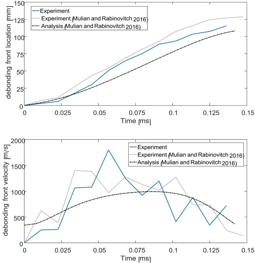
Figure 4: Debonding front kinematics: (a) location of the debonding front Vs. time; (b) velocity of the debonding front Vs. time. Time coordinate shifted to the initiation of the debonding process. Legend: — Experiment; ..... Experimental results in Mulian and Rabinovitch 2016; - - - - Numerical results in Mulian and Rabinovitch 2016.
