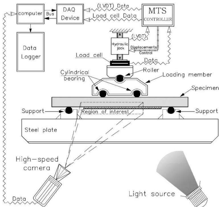
Figure 2 – Dynamic test setup (Mulian and Rabinovitch (2016))
