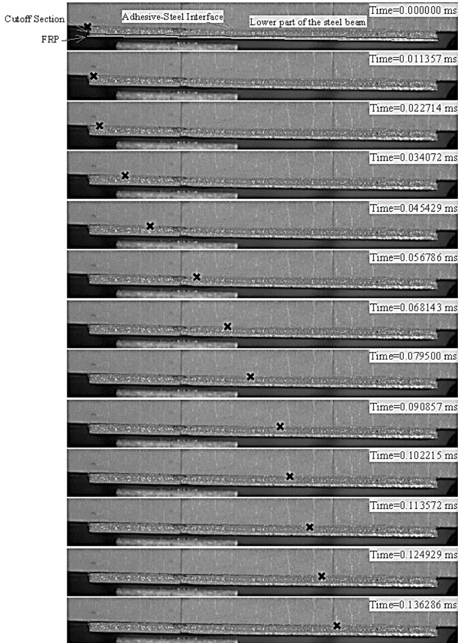
Figure 3: Debonding Front kinematics: A series of snapshots of the lower part of the beam, the adhesive layer and the FRP plate taken at intervals of  $11.36 \cdot 10^{-6}$  s during the debonding process. The cross marks designate the crack tip.
