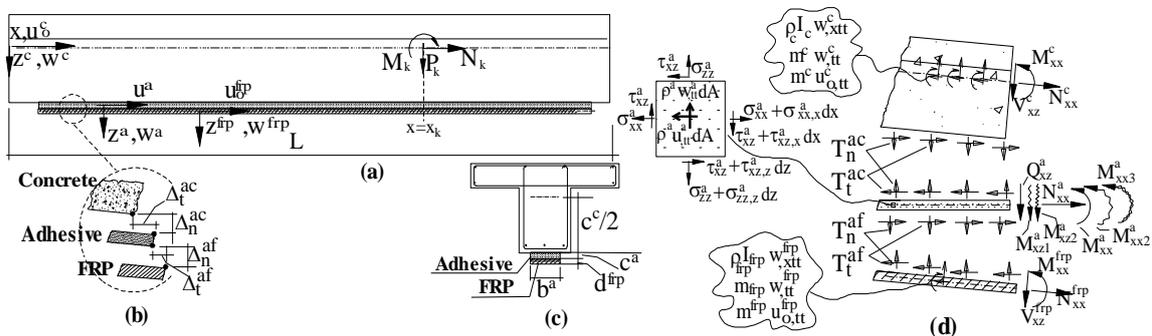
Figure 1: Notations and sign conventions (Rabinovitch 2014a): (a) Geometry and displacements; (b) cross section; (c) displacement jumps across the cohesive interfaces; (d) stress resultants, inertial effects, and dynamic equilibrium in the adhesive layer.
