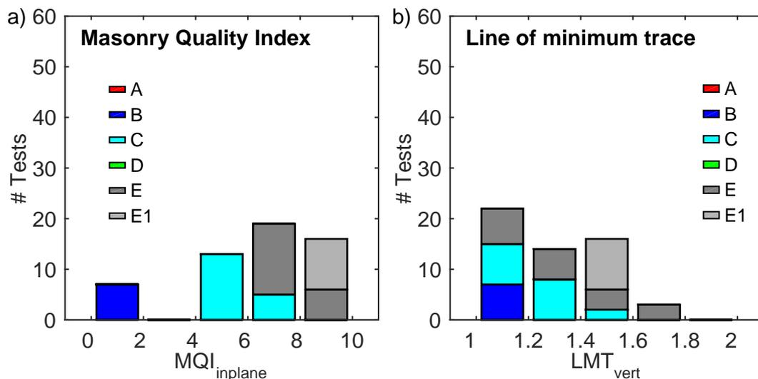
**Figure 6 Correlation between the masonry typology and the Masonry Quality Index (a) and the line of minimum trace (b) (Vanin et al. 2017).**
