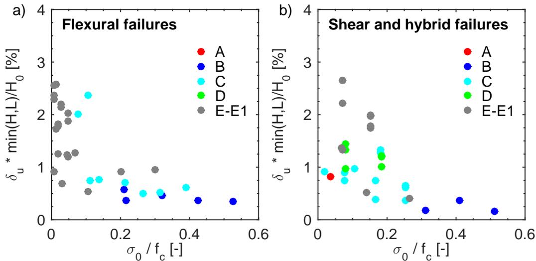
**Figure 7. Drift capacity as a function of the axial load ratio (Vanin et al. 2017).**
