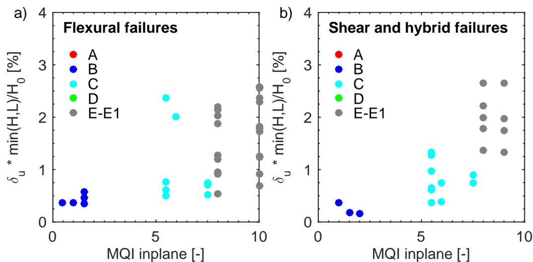
**Figure 8. Drift capacity as a function of the Masonry Quality Index.**
