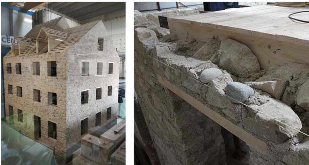
**Figure 3. Photos of the two buildings to be tested on the shake table at the Eucentre, Pavia, Italy. View of the entire structure and one structural detail showing a spandrel (Photos: I. Senaldi).**
