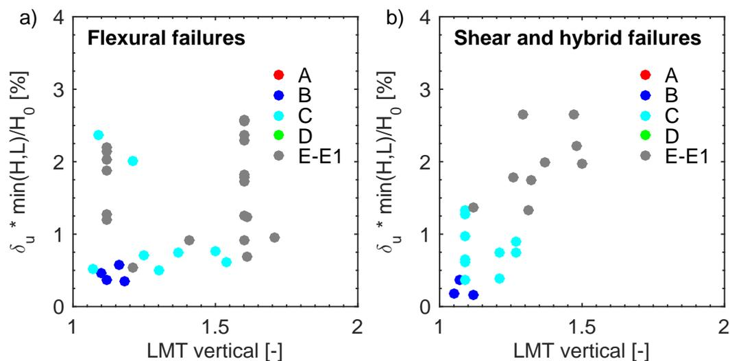
**Figure 9. Drift capacity as a function of the normalized length of minimum trace.**
