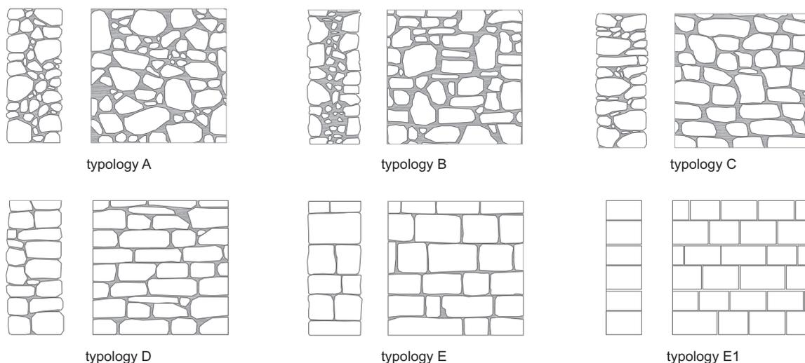
**Figure 5 Stone masonry typologies: sketches of typical textures and cross sections (Vanin et al. 2017).**
