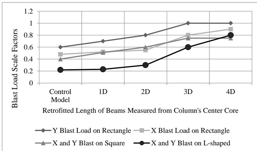
Figure 5. Shape effect on load carrying capacity of control and retrofitted frames.
