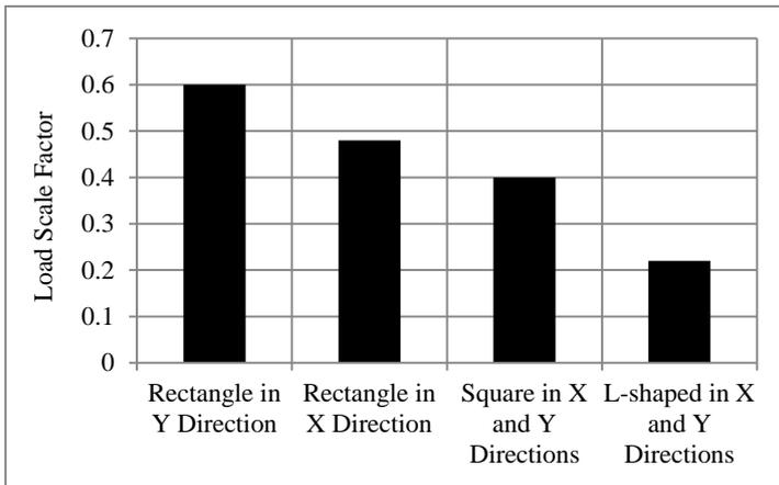
Figure 4. Load capacity of control frames with various shapes.
