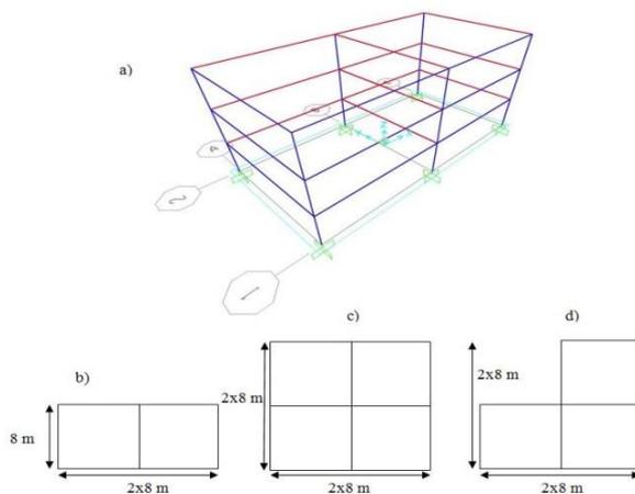
Figure 1. a) Base rectangular model with  $x$   $y$  and  $z$  coordinates b) plan view of rectangle c) plan view of the square model d) plan view of the L-shaped.
