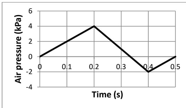
Figure 2. Air pressure wave of basic blast load (Jayashree et al. 2013).
