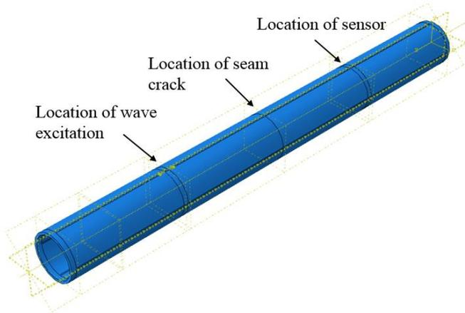
Figure 2 Location of actuator and sensor.
