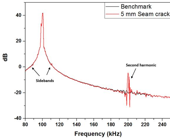
Figure 6 Received signal in the frequency domain with 1 ms input.
