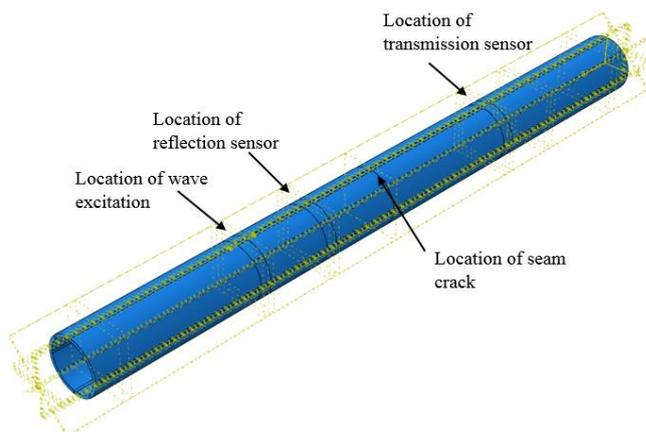
Figure 7 Simulation model of the steel pipe and the locations of actuator and sensors.
