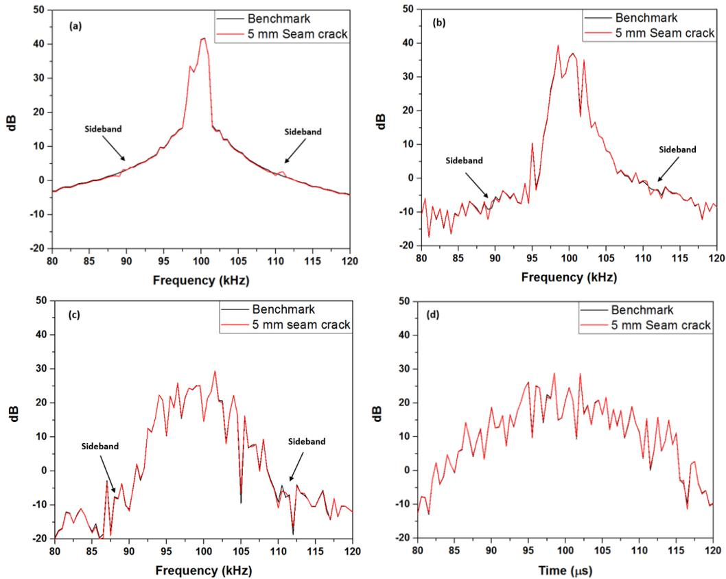
Figure 5 Received signal in the frequency domain (a) 1 ms input (b) 0.5 ms input (c) 0.2 ms input and (d) 0.1 ms input.
