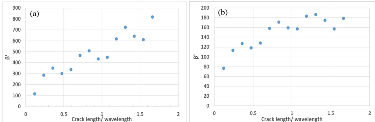
Figure 9 Nonlinear parameter  $\beta'$  in terms of crack length for (a) transmitted signal and (b) reflected signal.
