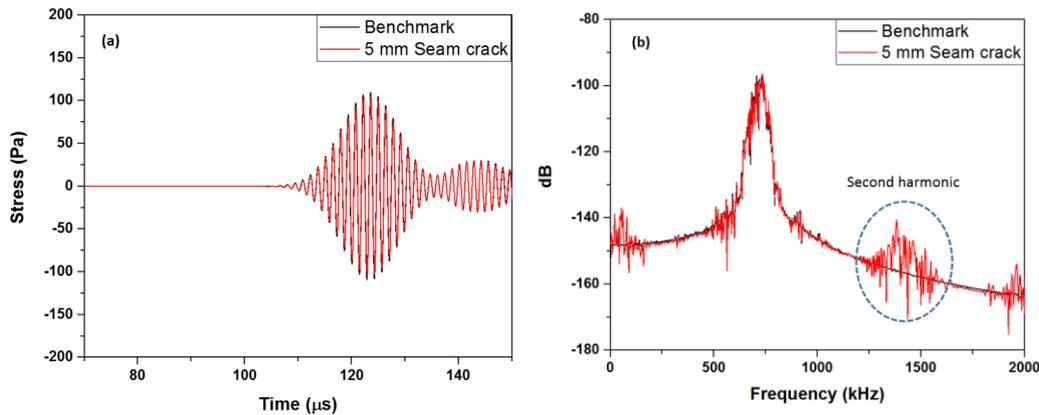
Figure 8 Transmitted signal in (a) time domain and (b) frequency domain
