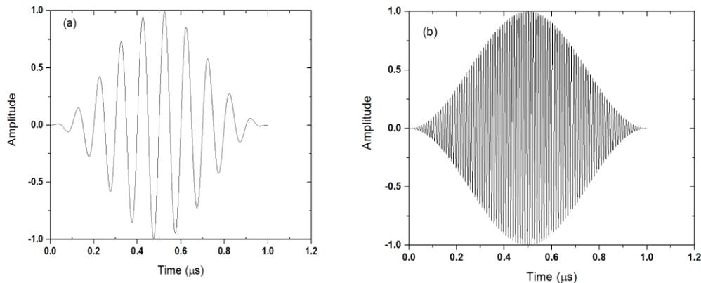
Figure 3 Input signal: (a) 1 ms (10 cycles) 10 kHz tone burst signal (b) 1 ms (100 cycles) 100 kHz tone burst signal.
