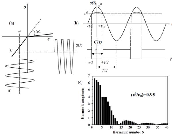
Figure 1 (a) Mechanical-diode" effect; (b) modulation of  $C(t)$ ; (c) high harmonic spectrum (Solodov, et al. 2010).
