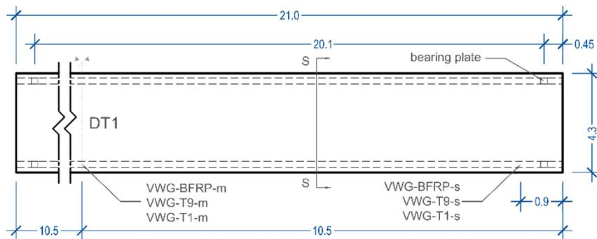
Figure 2. Plan view of the Double Tee 1 (measures in m).
