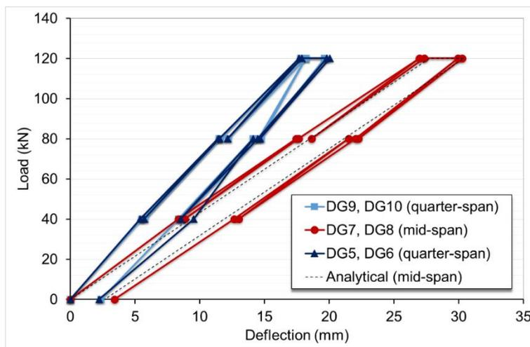
Figure 5: Load-Deflection diagrams.
