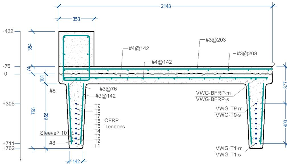
Figure 1. Cross section of the double tee with concrete topping and curb (measures in mm).
