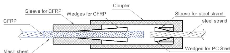
Figure 3. CFCC / PC strands anchorage system.
