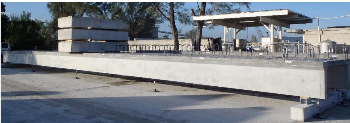
Figure 4. DT girder loaded under a three-point-load setup.
