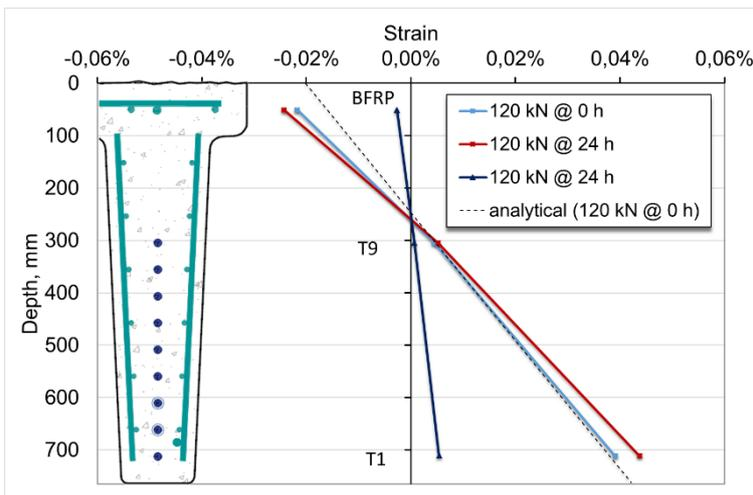
Figure 7: Measured strain profile at DT1 mid-span.
