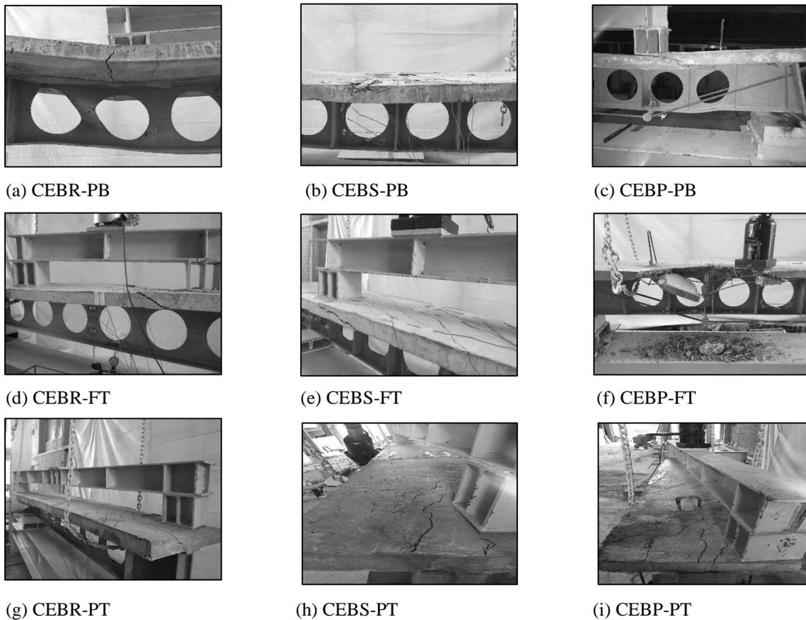
Figure 3. Failure modes of experimental specimens.
