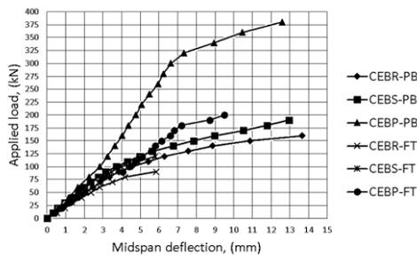
Figure 6. Load - midspan deflection of specimens.
