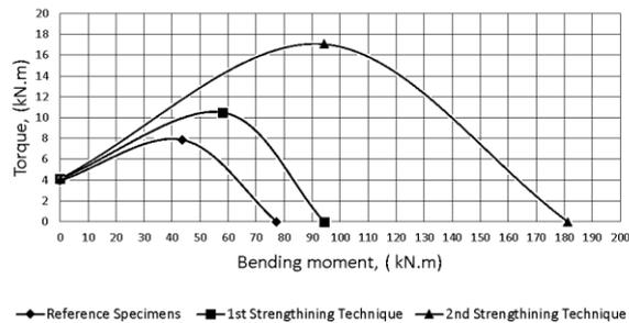
Figure 4. Flexure - torsion interaction diagram.
