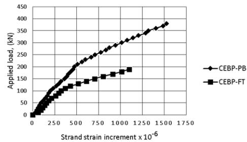
Figure 5. Load - strand strain increment diagram.
