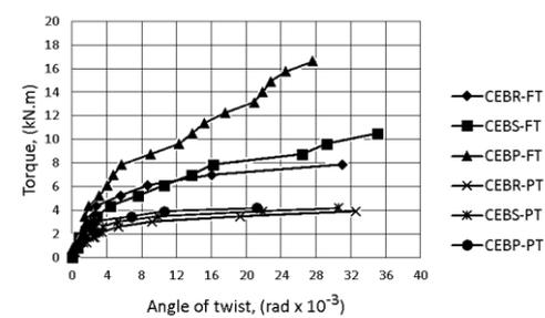
Figure 7. Torque - angle of twist of specimens.
