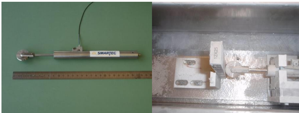
Figure 9. Fiber optic displacement sensor for ITER and cryogenic testing.
