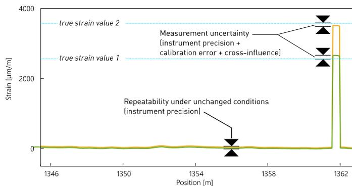
Figure 4. Distributed measurement data illustrating the definitions of uncertainty, accuracy, precision and repeatability
