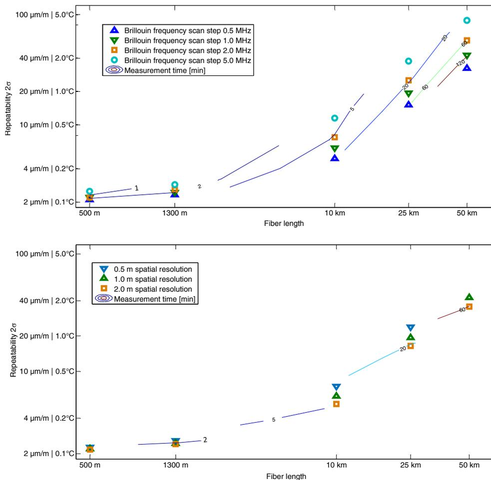
Figure 5: Repeatability and measurement times for a fixed spatial resolution of 1 m (*top*) and for a fixed Brillouin frequency scanning step of 1 MHz (*bottom*)
