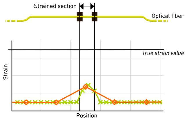
Figure 3. Definitions of spatial resolution and spatial accuracy for distributed strain sensing data in the case of a step-transition strain event
