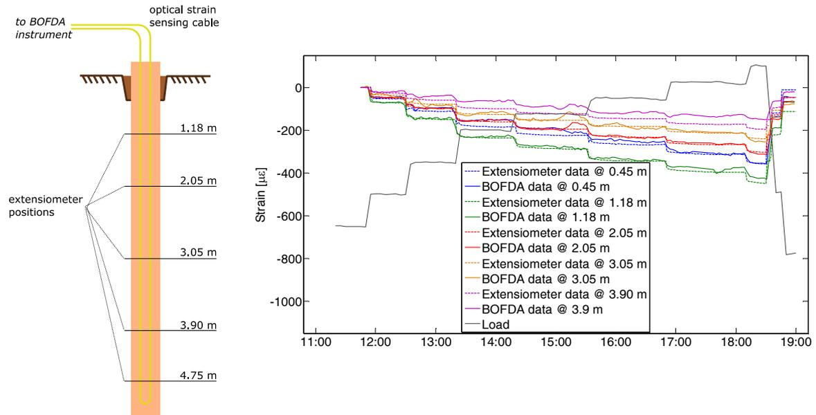
Figure 6: Set-up (*left*); Evolution of strain for both the extensometers and the distributed Brillouin sensors (at the exact extensometer positions, compensated for the base line reading at 0 kN load) over time (*right*).
