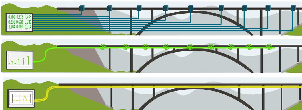
Figure 1. Schematic depiction of the definitions of discrete (*top*), quasi-distributed (*center*) and distributed (*bottom*) sensing points.
