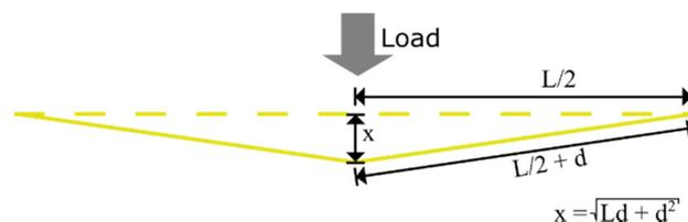
Figure 2. Measured strain based on the length change  $d$  of a distributed longitudinal sensor over a segment of length  $L$  due to a orthogonal load resulting in a displacement  $x$
