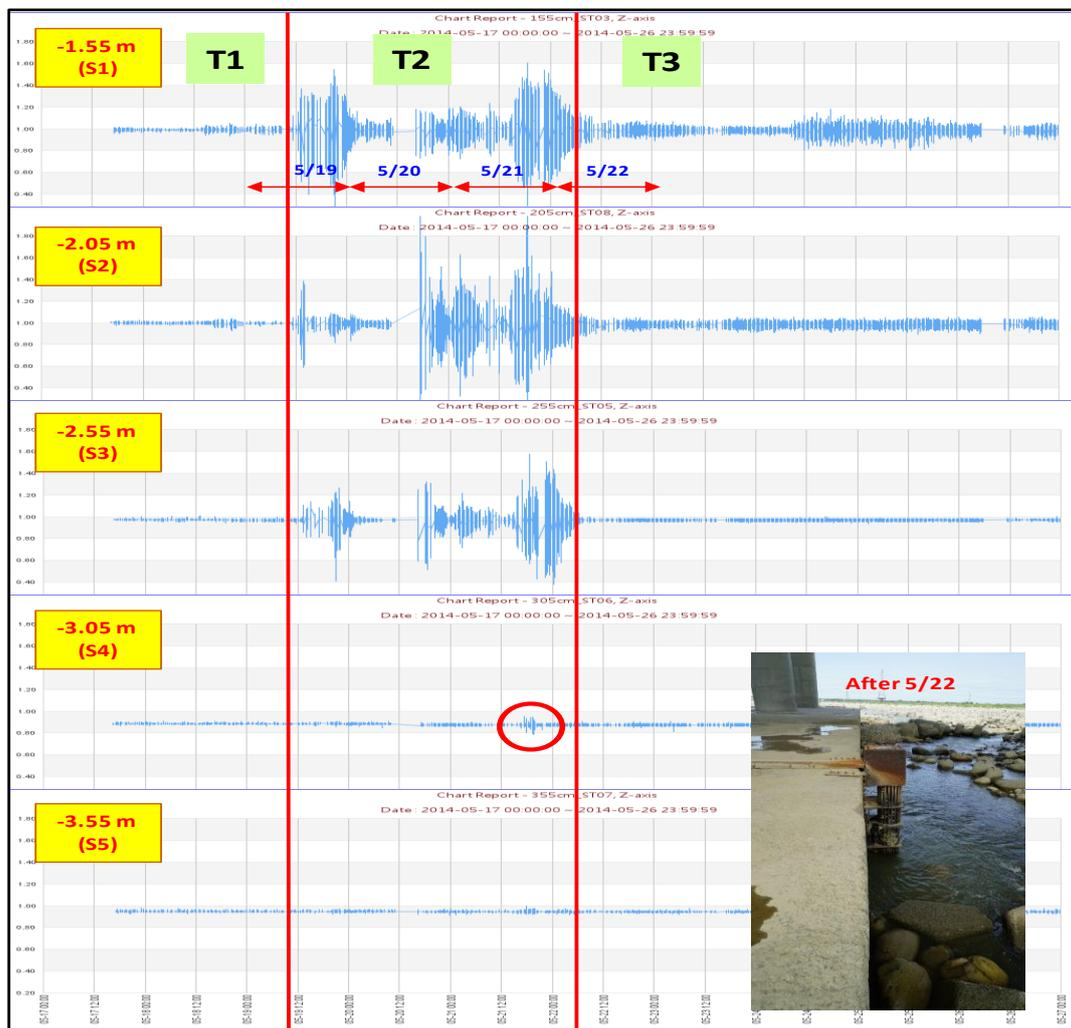
Figure 4 Responses of sensors during the scouring/deposition processes
