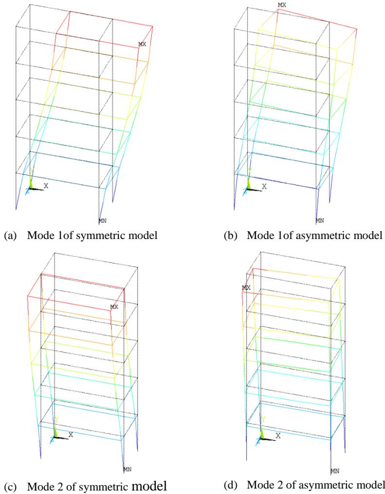
**Figure 2 Typical mode shapes of two models**
