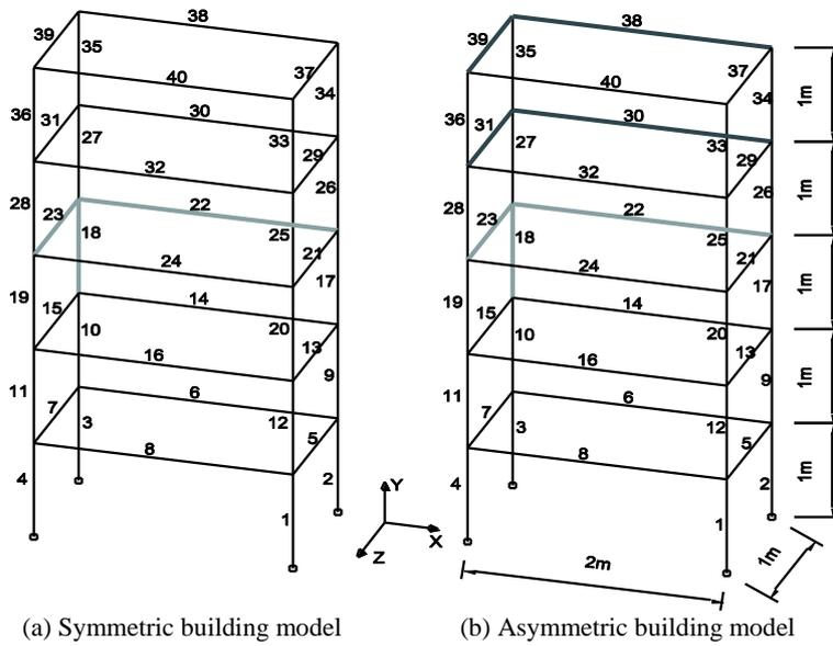
**Figure 1 3D Structural diagrams of two building models**
