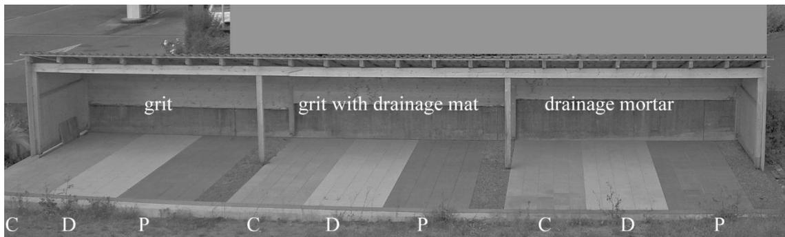
Figure 1: Overview of the facility. On three foundation types (grit, grit with drainage mat, and drainage mortar), we laid three different natural stone plates (C: Cresciano, D: Dietfurter, and P: Padang). The facility is partly sheltered and shows a 1.5% slope.
