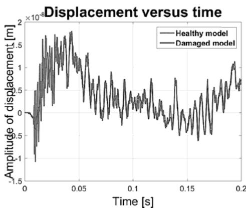
Figure 7: Displacement time histories for baseline and damaged states at point S1.
