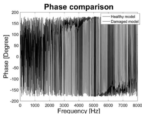
Figure 9: Phases of displacements in baseline and damaged states at point S1.
