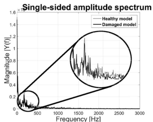
Figure 8: Single-sided amplitude spectra for baseline and damaged states at point S1.
