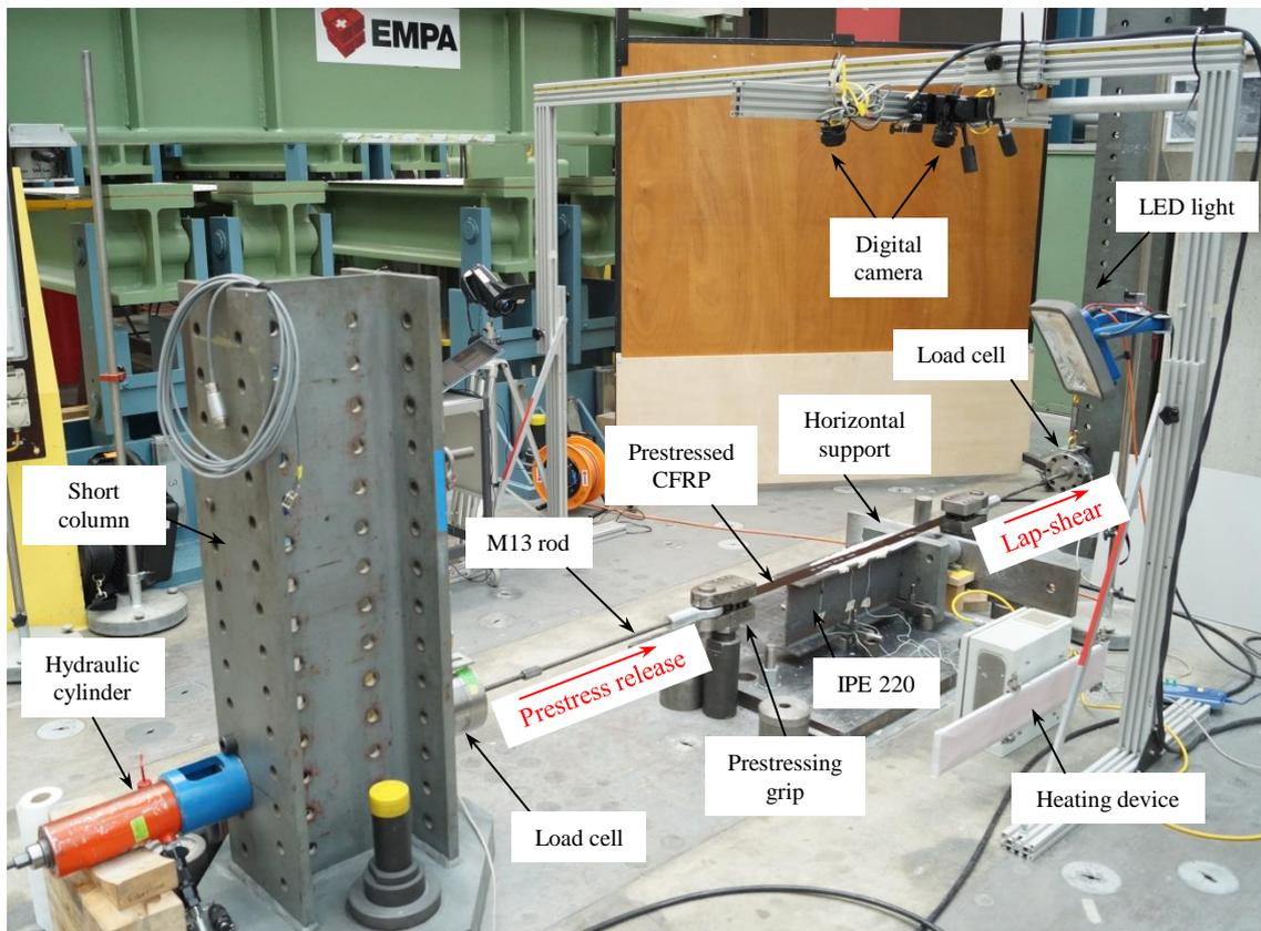
Figure 2. Lap-shear and prestress release test setup.
