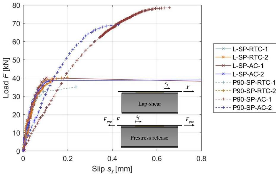
Figure 4. Load versus slip at the loaded end of tested specimens.
