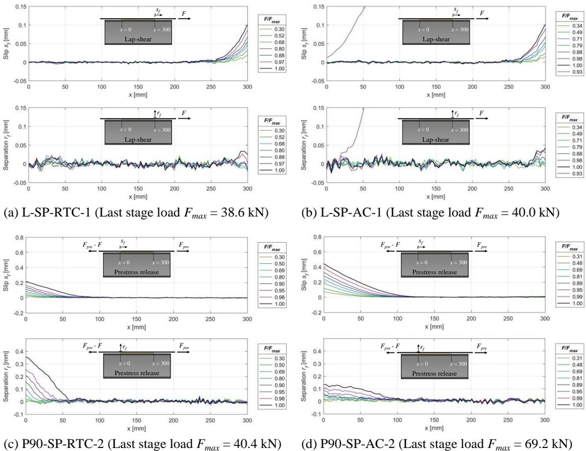
Figure 5. Evolution of in-plane and out-of-plane deformation profiles during loading ( $s_f$  = slip;  $r_f$  = separation).
