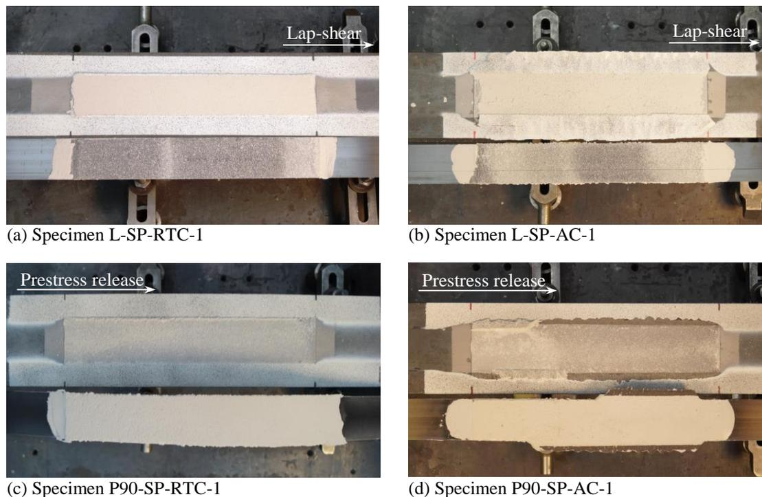
Figure 3. Failure modes observed in the tested specimens.
