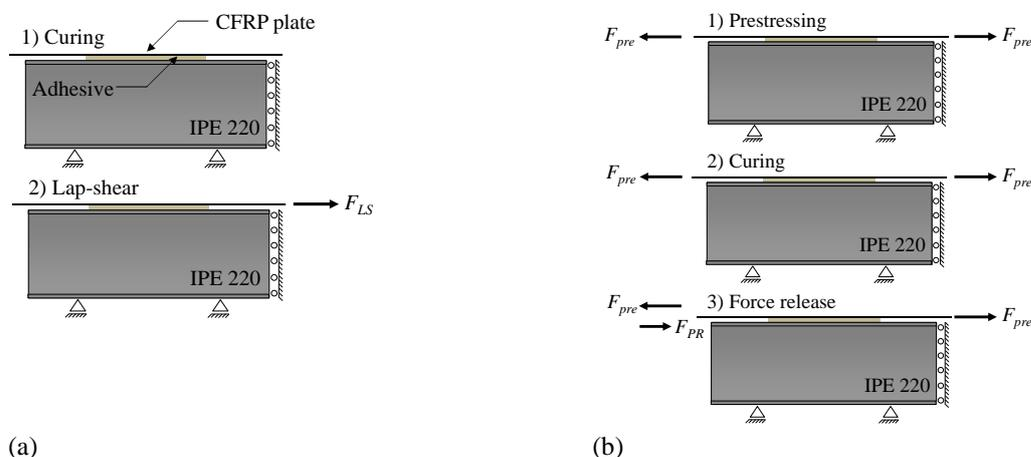
Figure 1. Procedure of: (a) lap-shear test; (b) prestress release test.
