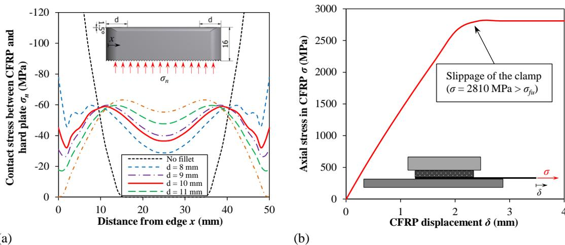
Figure 3. FE results: (a) effect of fillet dimension on the distribution of the contact pressure ( $d$  = fillet dimension); (b) ultimate capacity of the joint before slippage of the clamp.
