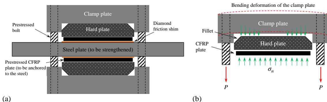
Figure 1. Schematic view of the mechanical clamping system: (a) cross-sectional view; (b) stress transfer between different parts.
