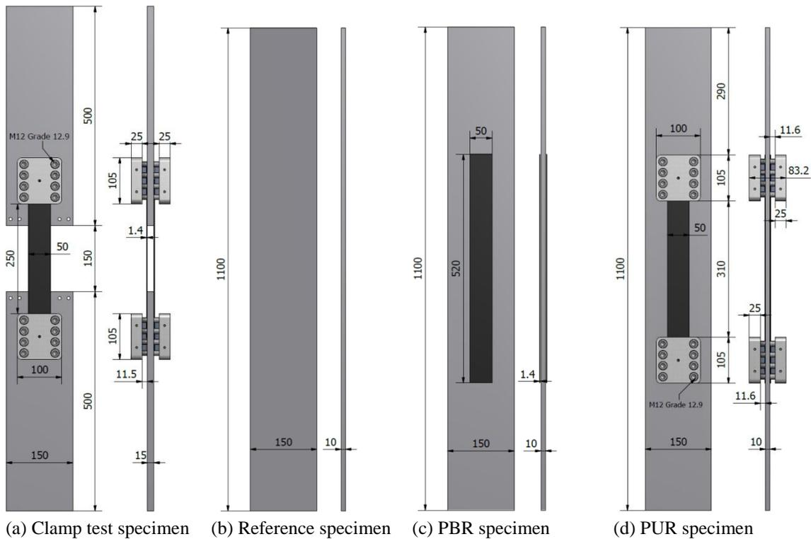
Figure 4. Tensile test specimens (all dimensions are in mm).
