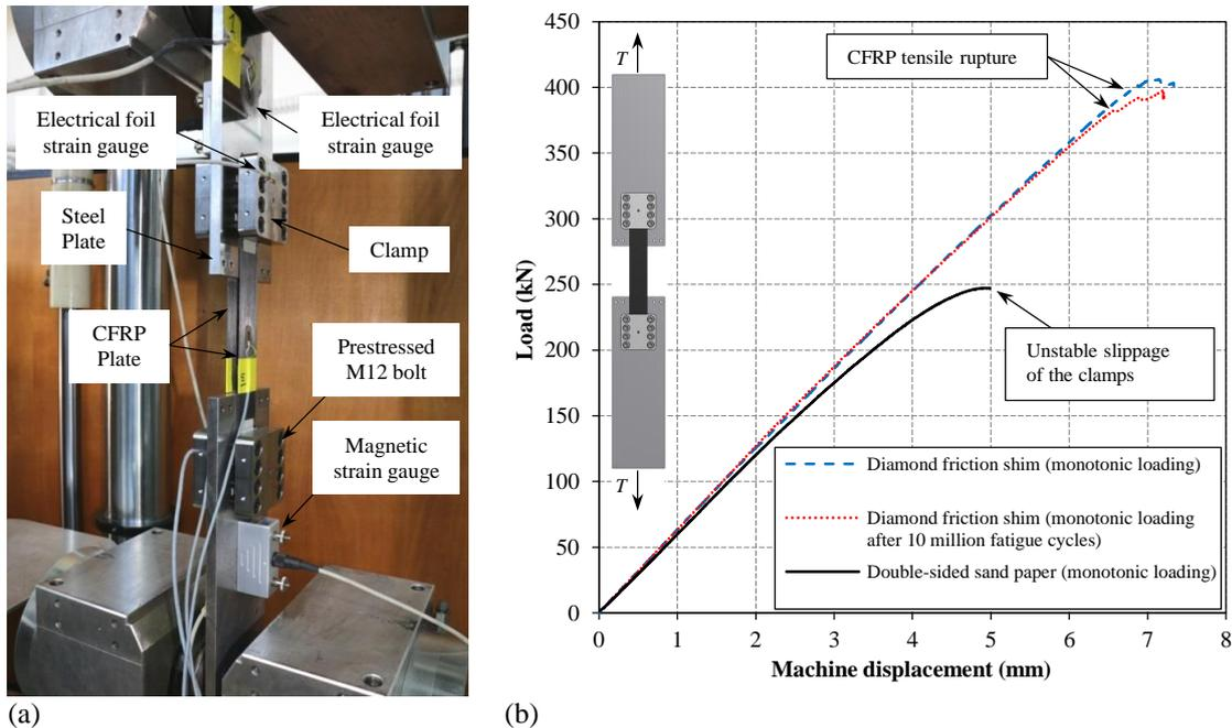
Figure 5. (a) Test setup for static and fatigue tests; (b) load–displacement response of clamp test specimens.
