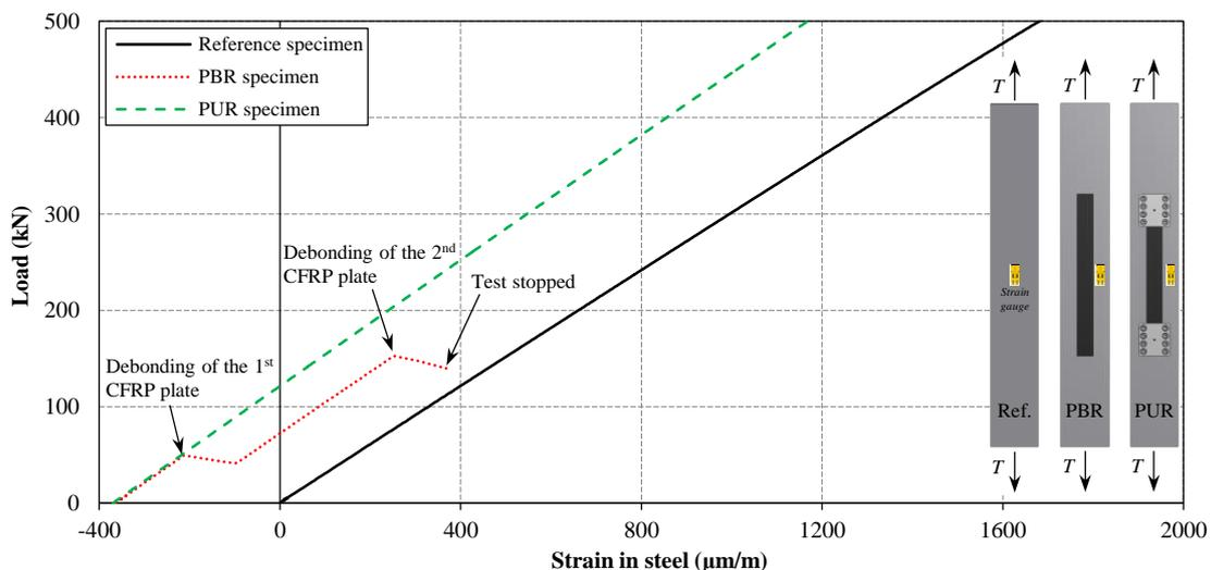
Figure 7. Load-strain response of the unstrengthened and CFRP-strengthened steel plate specimens.
