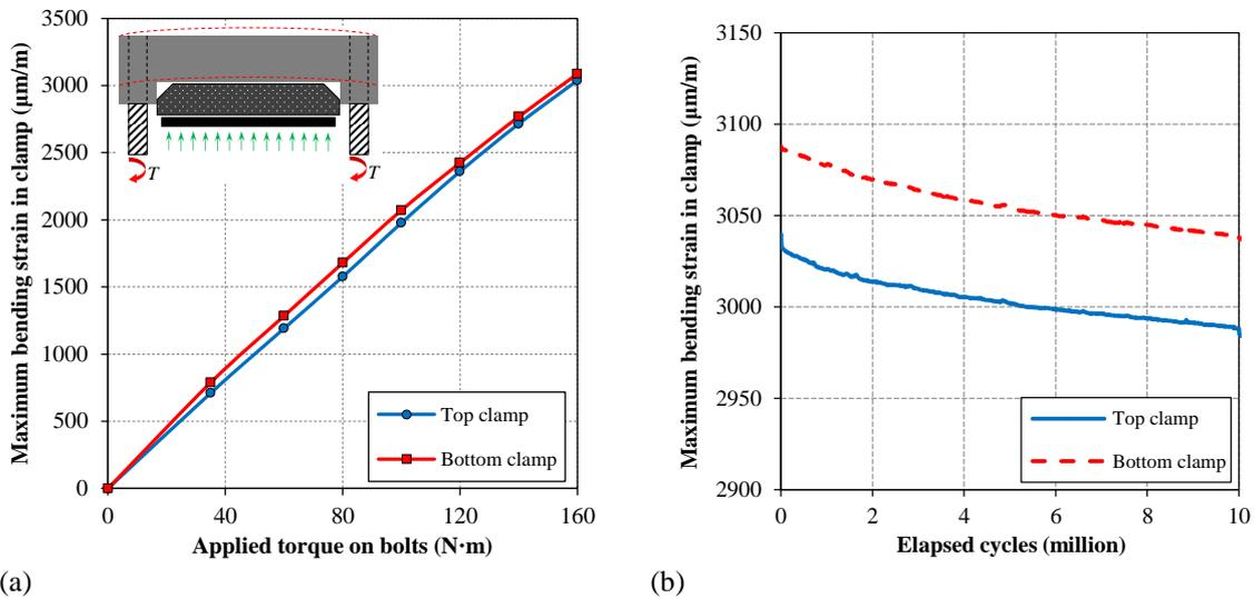
Figure 6. (a) Maximum bending strain in clamp plates versus applied torque; (b) evolution of maximum bending strain in mechanical clamps with respect to fatigue cycles.
