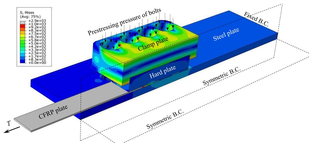
Figure 2. ABAQUS model of the mechanical clamping system for unbonded CFRP-to-steel joints.
