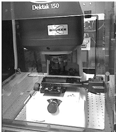
Figure 4. Laser profilometry for CFRP surface after failure analysis.
