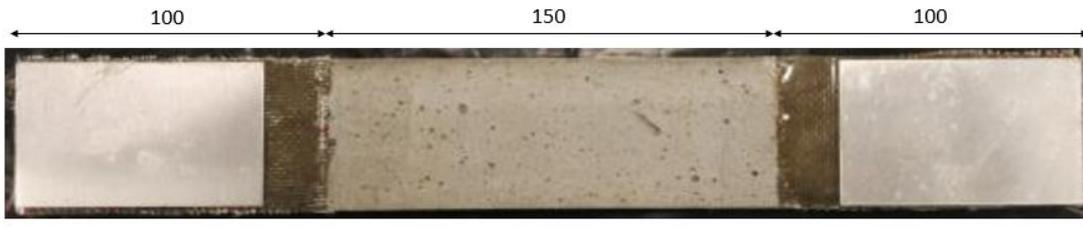
Figure 1. Configuration of strengthened specimen.
