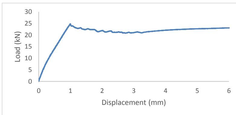
Figure 4. Typical load-displacement curve for 150mm bond length.
