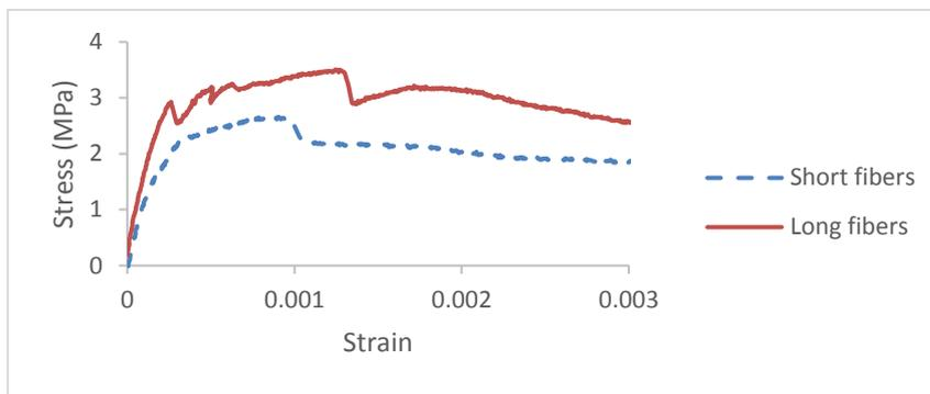
Figure 2. Typical test results for direct tensile test.
