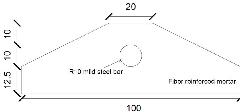
Figure 3a. Geometry of specimen, cross section of repair patch.
