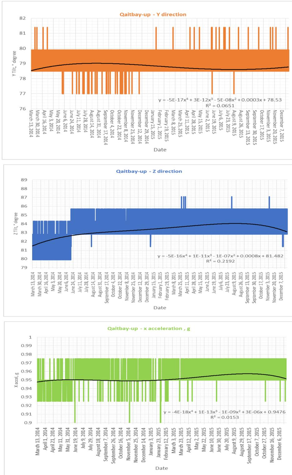
Figure.2 Tilt and acceleration results extracted from upper sensor located at Qaitbay minaret
