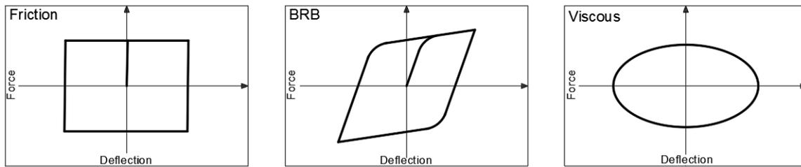
Figure 4. Idealized force-displacement relationship of passive dampers
