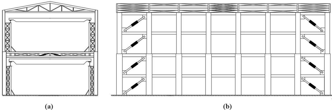
Figure 5. Location of viscous damper. a) Devices used to reduce cranes vertical vibration, b) Devices used to reduce the response of building due to earthquake excitation.
