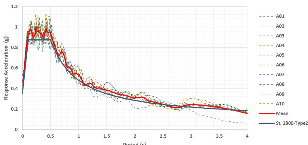
Figure 3. Acceleration response spectrum of Iranian national seismic code and the artificial accelerograms.
