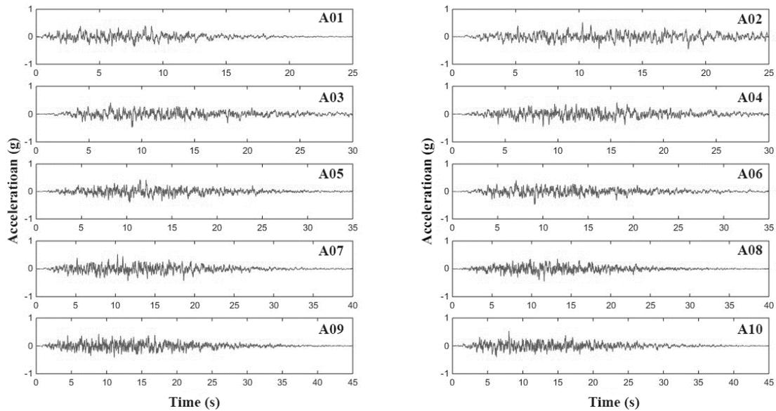
Figure 2. Acceleration time series of randomly generated earthquake.
