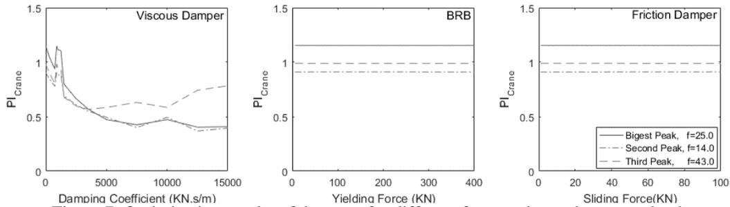
Figure 7. Optimization results of dampers for different frequencies under cranes load.
