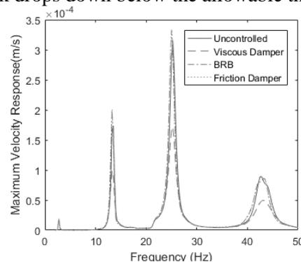
Figure 10. Velocity response frequency spectrum of floor deck with and without damper
