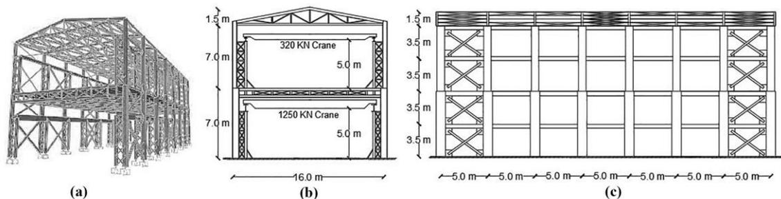
Figure 1. Industrial building shape and dimensions, a) 3D view, b) Cross section, c) Longitudinal view.
