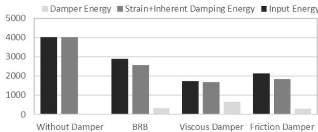
Figure 9. Input seismic energy and its distribution in the building for different types of dampers.
