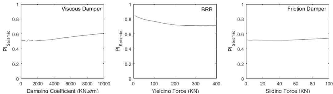
Figure 6. Optimization results of dampers for seismic loading.
