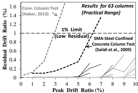
Figure 5. Residual drifts for all practical SMA-reinforced FRP-confined concrete columns.
