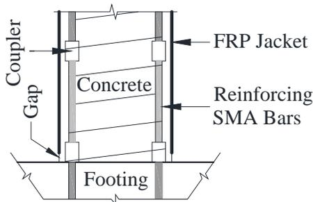
Figure 1. Plastic Hinge Detail for Proposed Columns.
