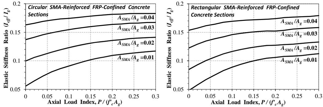
Figure 2. Effective Moment of Inertia for SMA/FRP Columns.
