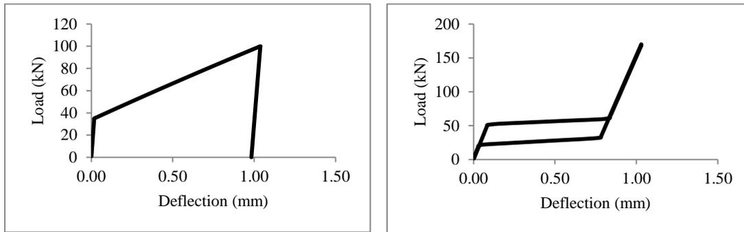
Figure 4. Load bearing capacity of plates (i) Load deflection curve for steel plate after loading unloading cycle (ii) Load deflection curve for Ni-Ti SMA plate after loading unloading cycle
