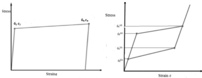
Figure 1. Material models for Steel (kinematic hardening) and Superelastic SMA (SE)
