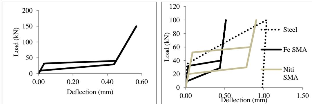
Figure 5. Load bearing capacity of plates (i) Load deflection for ferrous SMA plate after loading unloading cycle (ii) Comparative curve of load deflection for all plates with different material after loading unloading cycle
