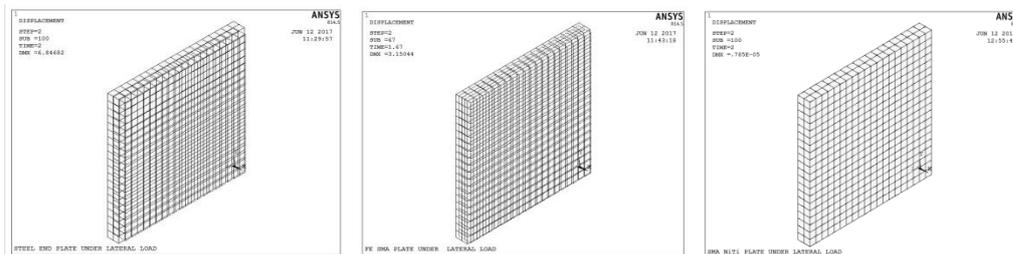
Figure 3. Deflection of plates under lateral load (i) Steel plate, (ii) Ferrous SMA plate, (iii) Ni-Ti-SMA plate
