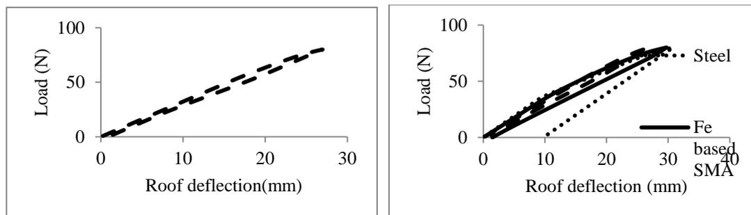
Figure 8. Load bearing capacity of frames (i) Load deflection for frame with Ni-Ti SMA end plate for loading unloading cycle (ii) Comparative load deflection of all frames with different material end plates for loading unloading cycle
