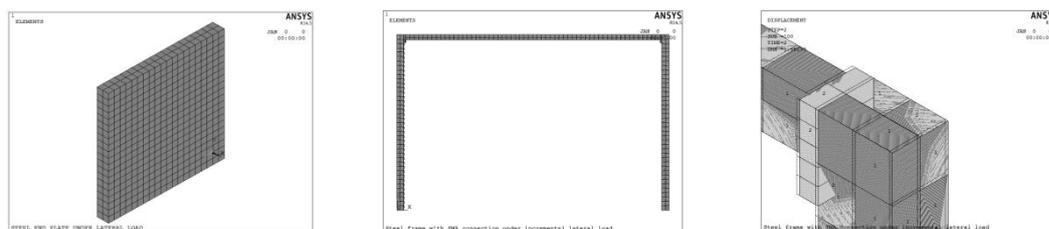
Figure 2. Finite element model (i) Plate, (ii) Simple frame, (iii) Ferrous SMA at connection
