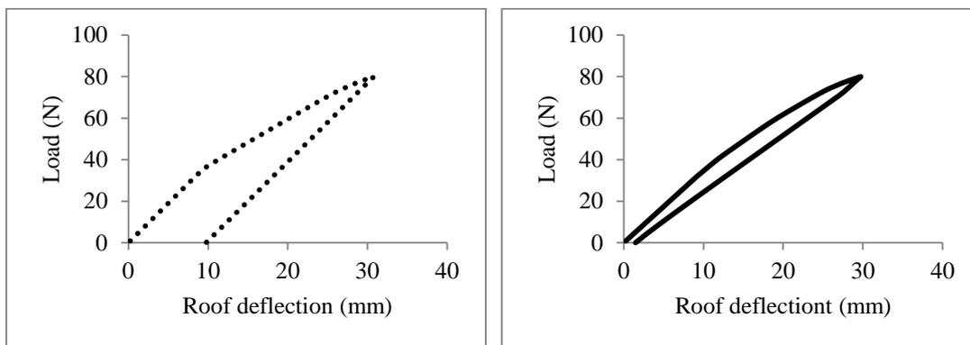
Figure 7. Load bearing capacity of frames (i) Load Deflection for frame with steel end-plate for loading unloading cycle (ii) Load deflection for frame with ferrous SMA end plate for loading unloading cycle
