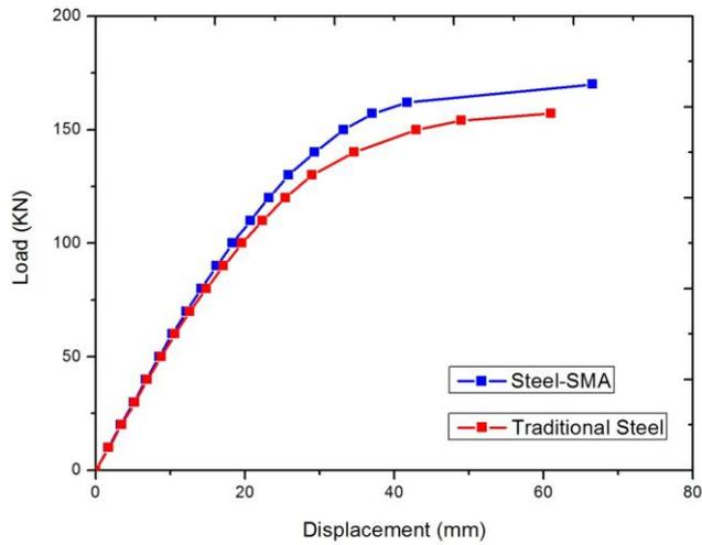
Figure 5: Load – Deflection curve of beam-column joints
