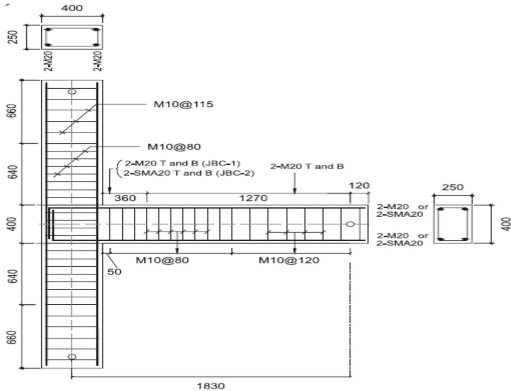
Figure 1: Reinforcement details of specimens JBC-1 and JBC-2 (all dimensions are in mm)
