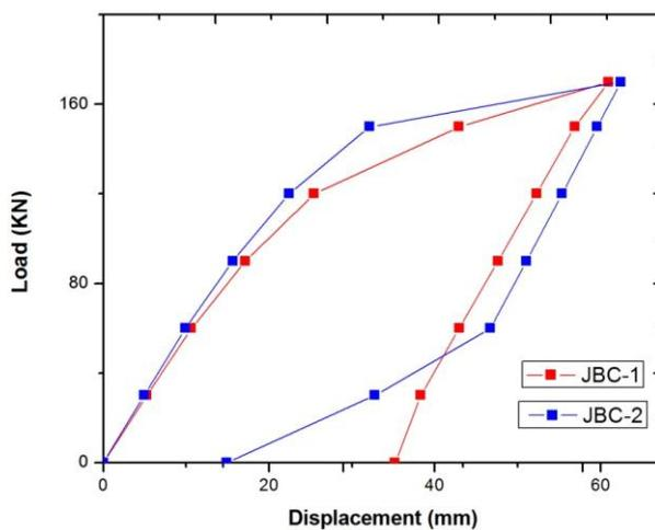
Figure 6: Numerical mid-span displacement versus load graph
