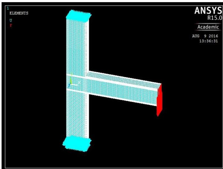
Figure 4: Loading and Boundary condition
