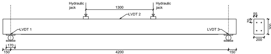
Figure 1. Beam specimens under four-point bending test
