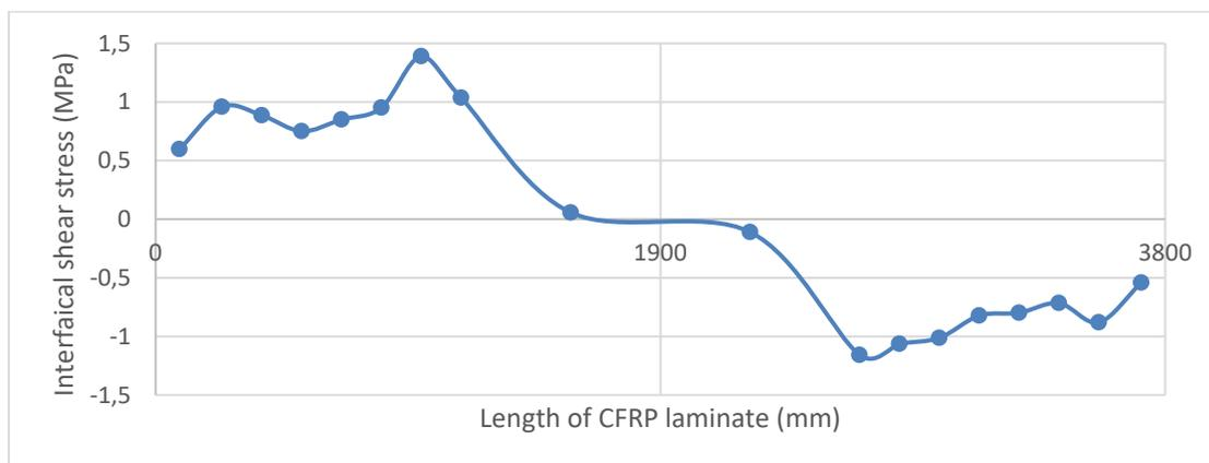
Figure 5. Interfacial shear stress between CFRP laminate and concrete beam under prestressing force of 80 kN in specimen B3
