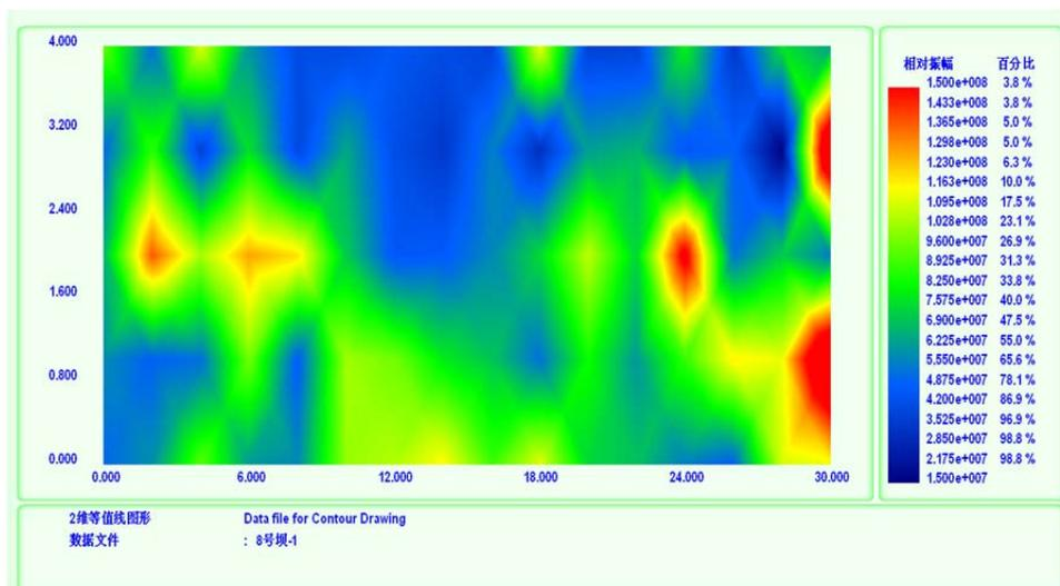
Figure 7 Isopleths Distribution Diagram of FBT Deformation Modulus (15MPa-150MPa)
