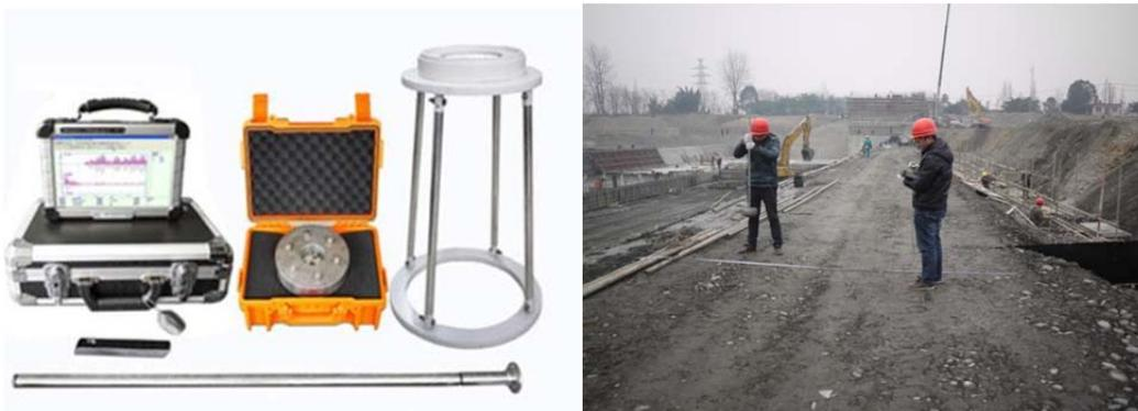
Figure 4: Falling Ball Geomechanics Test Instrument (SEH-FBT) Figure 5: Field Test
