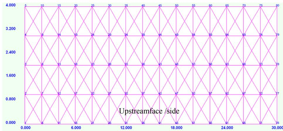
Figure 6: Distribution Figure of Falling Ball Test
