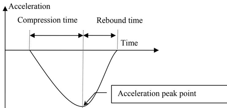
Figure 3: Separations of Compression and Rebound Process
