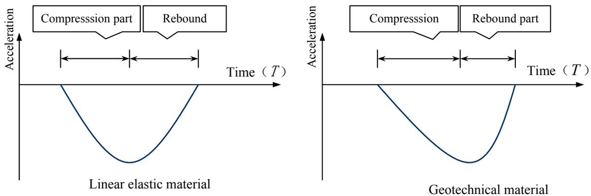
Figure 2: Compression Process and Rebound Process after the Fall Ball Contact
