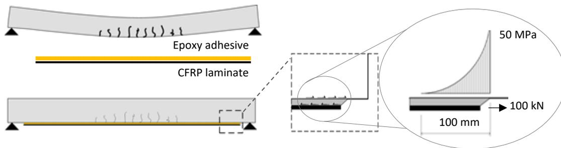
Figure 2. Interfacial shear stress concentration developed at each end of CFRP laminate upon releasing of prestressing force (Haghani and Al-Emrani, 2016; Haghani et al., 2009)
