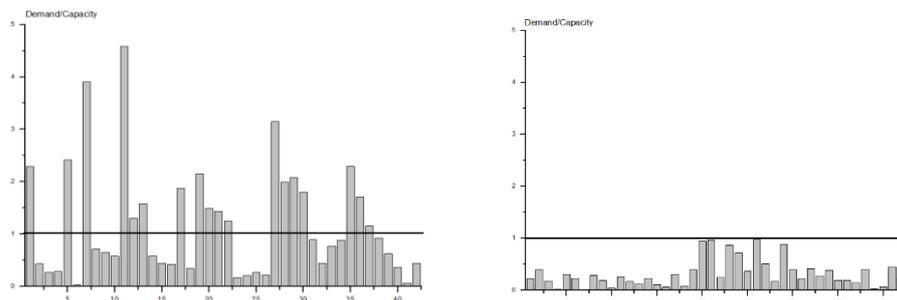
Figure 12. a) Demand/Capacity relation in pedestal, in the critical direction (transverse) of structure without rehabilitation, b) Demand/Capacity relation in pedestal, in the critical direction (transverse) of structure with rehabilitation, using SL-B devices.
