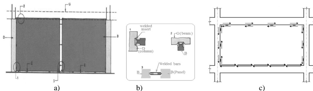
Figure 5. a) Dispositions of the inserts on structural elements, b) Detailed of the joints between shear walls and walls-frame, c) Shear walls behavior in the Girón system.
