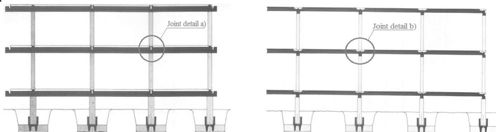
Figure 2. Typical structural sections of Giron System. a) Frames in the beam direction (transverse frame), b) Frames in the direction of the double T slab (longitudinal frame).
