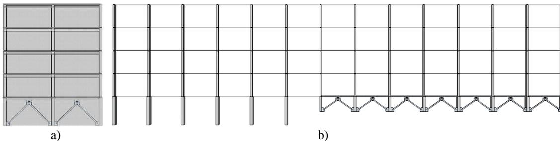
Figure 8. a) Solution to strengthening shear walls capacity, b) Solution to avoid weakness of the structural first floor.
