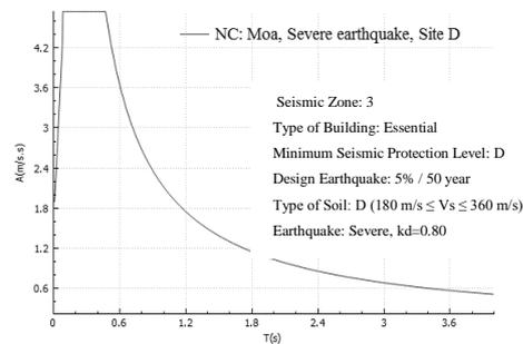
Figure 6. a) Earthquake Hazard, oriental zone of Cuba, and Geographical area of the Moa site where the hospital is located, b) Earthquake design defined in terms of Elastic Response Spectrum for the Cuban Seismic Standard, NC 46:2013 for the Moa City.
