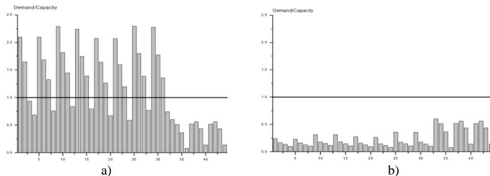
Figure 11. a) Demand/Capacity relation in shear walls in the critical direction (longitudinal) of structure without rehabilitation, b) Demand/Capacity relation in shear walls in the same direction (longitudinal) of structure with rehabilitation using SL-B devices.
