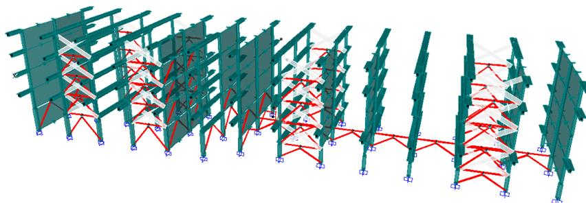
Figure 9. Schemes with the definitive positions of the devices SLB used in the building.
