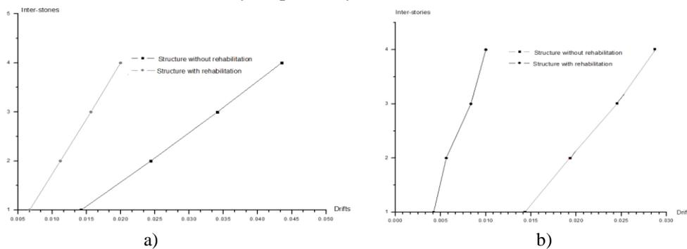
Figure 10. a) Drifts of the structure in transverse direction, b) Drifts of the structure in longitudinal direction
