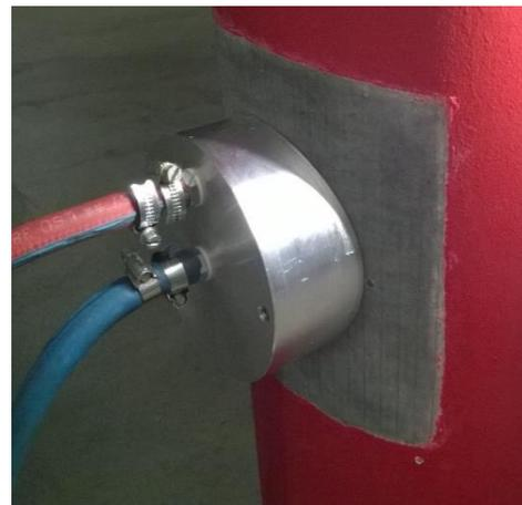
Figure 8. Project B, permeability measurement on column,
