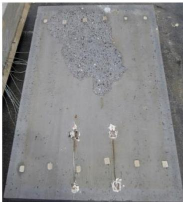
Figure 5. Initial spalling occurred in the test after 14 minutes.
