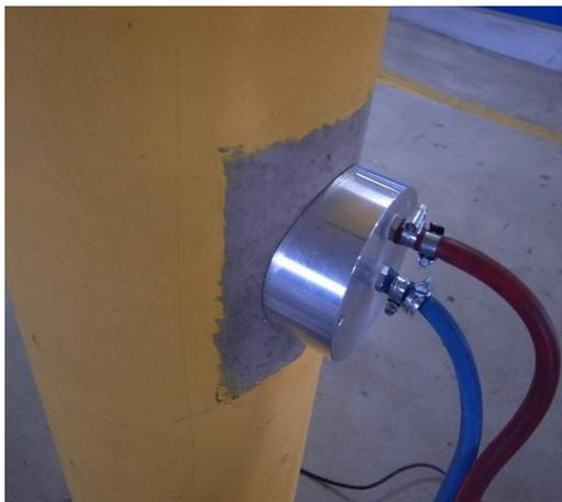
Figure 7. Project A, permeability measurement on column.
