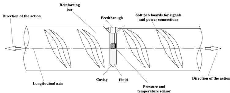
Figure 1. Longitudinal section of the system.
