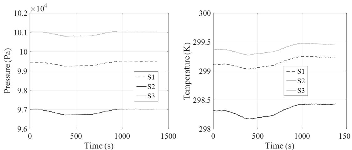
Figure 4. Pressure and temperature variations during the loading and unloading cycle.
