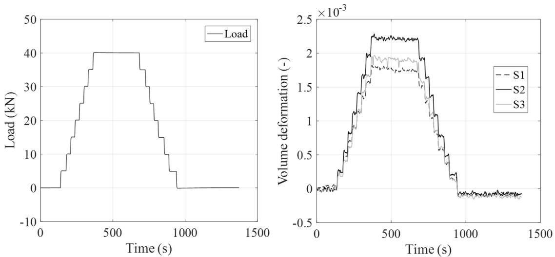
Figure 5. Axial load and total volume deformations during the loading and unloading cycle.
