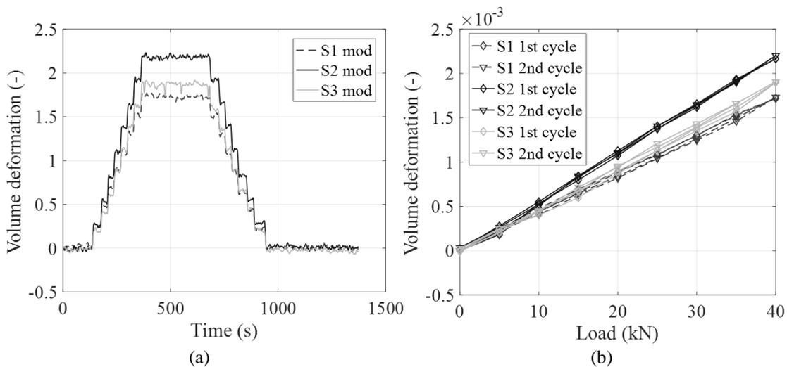
Figure 6. Corrected volume deformations as a function of either time (a) or the applied axial load (b).
