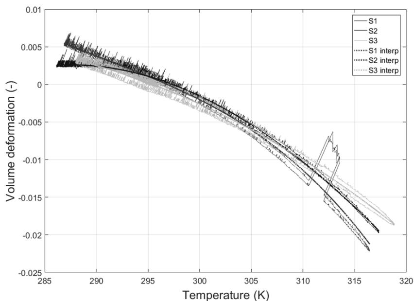
Figure 3. Temperature calibration for the three measuring units.
