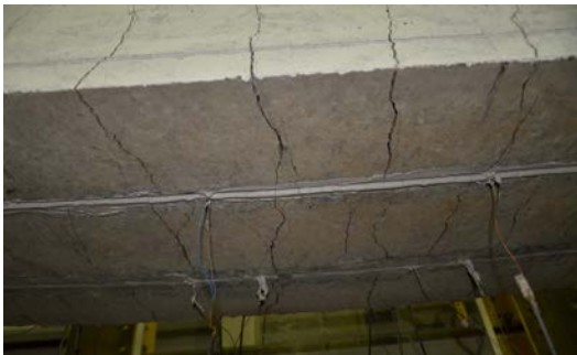
Figure 8. Crack pattern on the bottom surface of beams series B: (a) NSM12B, (b) NSM12BL.
