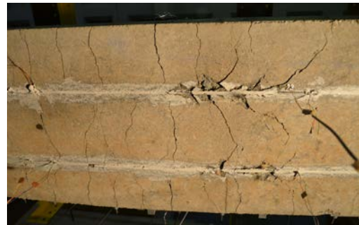
Figure 8. Crack pattern on the bottom surface of beams series B: (a) NSM12B, (b) NSM12BL.
