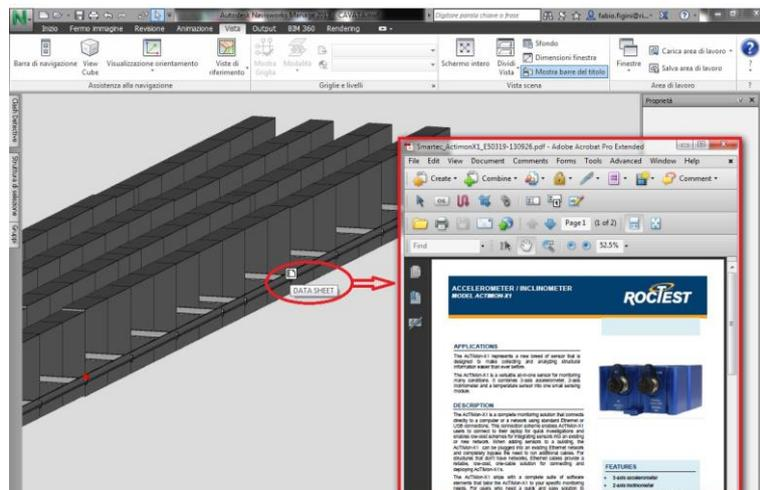
Figure 7. Visualization of sensor data sheet.
