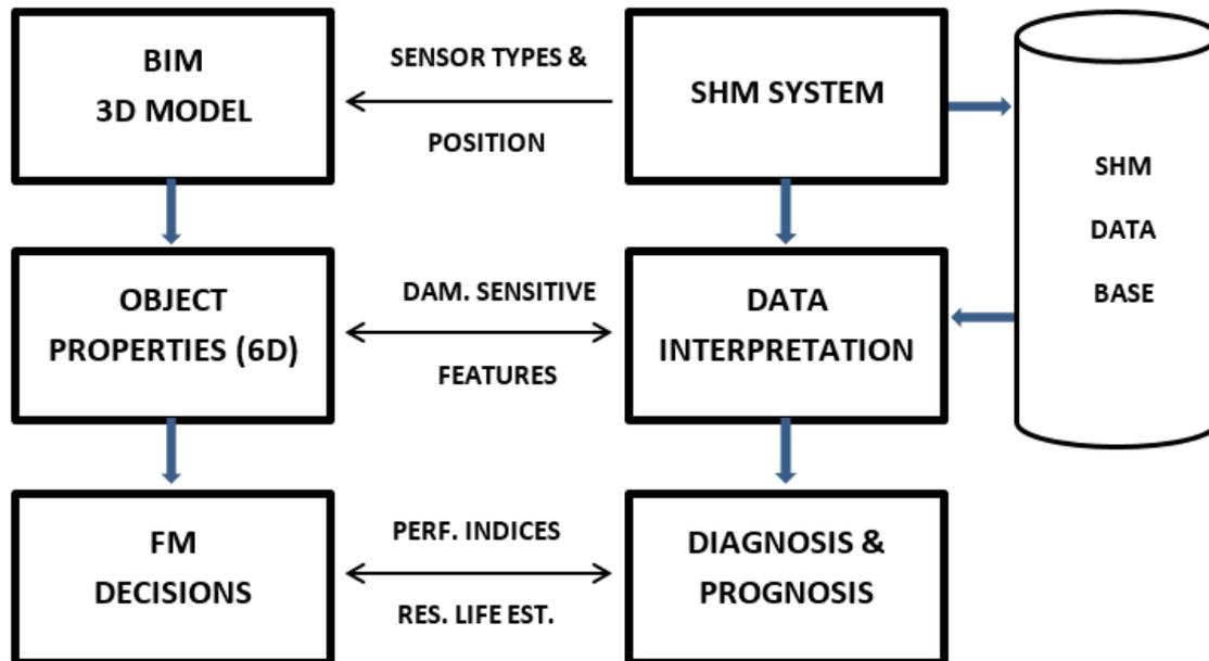
Figure 2. Complete process representation.
