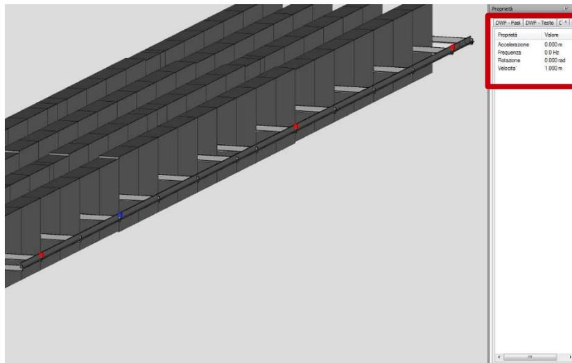
Figure 6. Visualization of sensors (red, blue points) and shared parameters values from Revit (red box).
