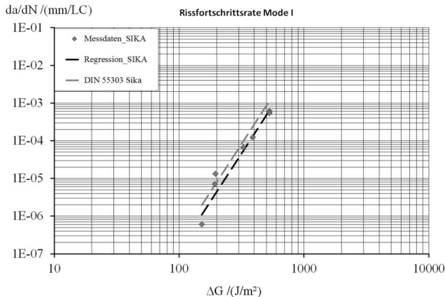
Figure 3. Crack propagation rate of the highly toughened adhesive measured under dynamic DCB loading on GRE substrates.
