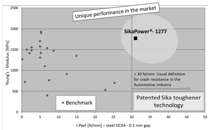
Figure 1. E-modulus vs I-Peel of different 2C epoxies adhesives. ♦commercially available products, ■ final product SikaPower®-1277.
