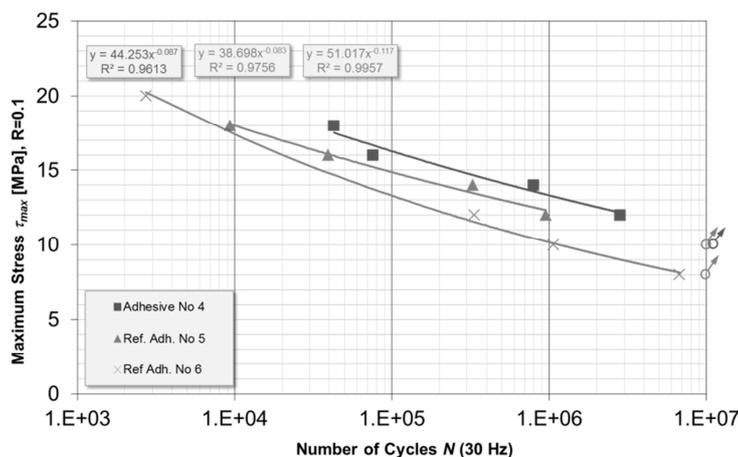
Figure 2. Dynamic lap shear strength fatigue on GRE substrates using x non-toughened adhesive, ▲ medium toughened reference adhesive, ■ highly toughened adhesive.
