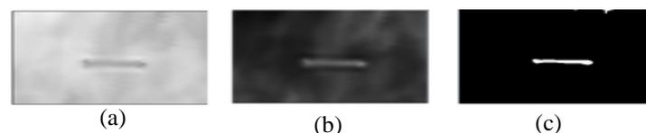
Figure 9. Images of notch 1 under the 2-mm thick rubber layer obtained at standoff distance of 0.1 mm.: (a) original and after (b) average filtering and (c) thresholding by the developed fuzzy c-mean thresholding algorithm.
