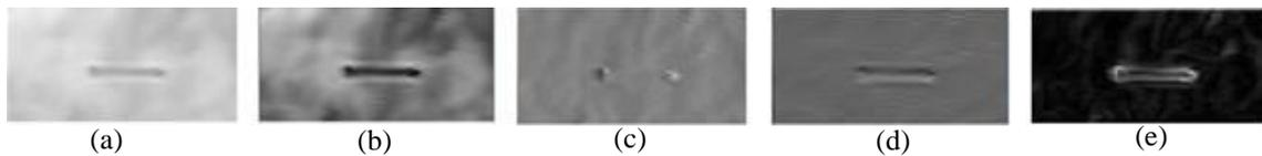
Figure 7. Images of notch 1 under the 2-mm thick rubber layer obtained at standoff distance of 0.1 mm: (a) original and after (b) average filtering, (c) gradient filtering in x direction ( $G_x$ ), (d) gradient filtering in y direction ( $G_y$ ) and e) gradient magnitude with Sobel method,  $|G| = \sqrt{G_x^2 + G_y^2}$ .
