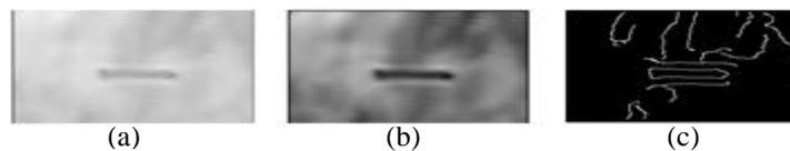
Figure 8. Images of notch 1 under the 2-mm thick rubber layer: (a) original and after (b) average filtering, (c) canny edge detection algorithm obtained at standoff distance of 0.1 mm.
