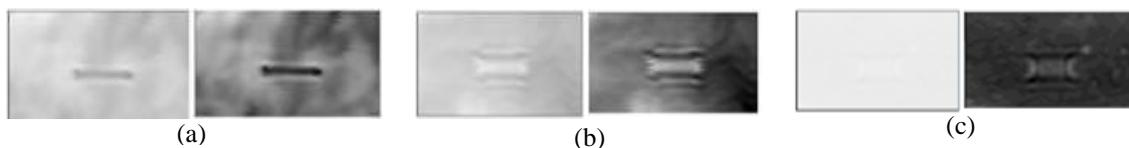
Figure 5. Original (left) and enhanced (right) images of notch 1 under the 2-mm thick rubber layer obtained at three standoff distances: (a) 0.1mm, (b) 0.25 mm and (c) 4 mm.
