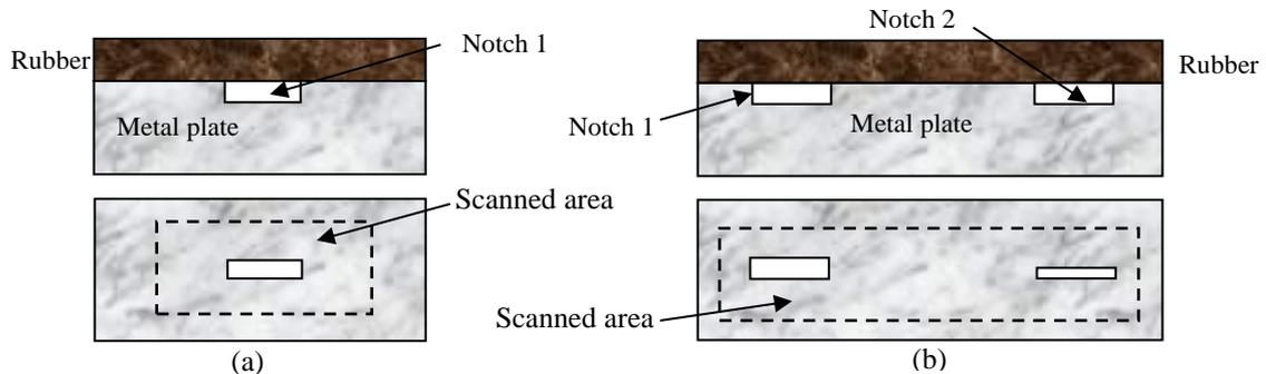
Figure 1. Cross-sectional side view (upper) and schematic of the top view without rubber layer (lower) of the parts of aluminum plate with (a) notch 1 and (b) notches 1 and 2.
