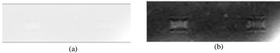
Figure 6. (a) Original and (b) enhanced images of notches 1 and 2 under the 4-mm thick rubber layer obtained at standoff distance of 0.1 mm.
