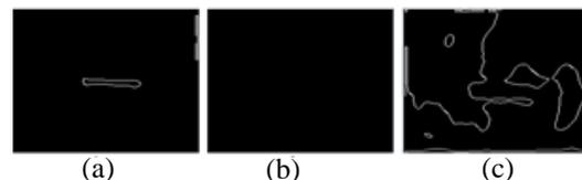
Figure 11. Notch edge detection obtained with a) the developed fuzzy c-mean thresholding algorithm, b) traditional fuzzy c-mean thresholding algorithm and c) Otsu's thresholding algorithm.
