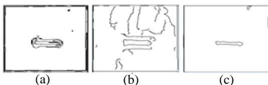
Figure 10. Notch edge detection obtained with the a) gradient magnitude using Sobel's gradient, b) Canny edge detection algorithm and c) developed fuzzy c-mean thresholding algorithm.
