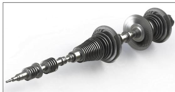
Figure 5: Final 3D CAD of the complete steam turbine.
