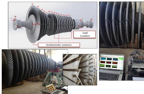
Figure 8: Schematic illustration of the measurement geometry and real experimental set-up for the modal analysis of the intermediate pressure rotor.
