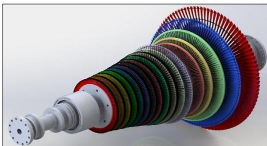
Figure 4: Complete 3D CAD assembly of the intermediate pressure section, including the rotor shaft and the blades of all the 17 sections.
