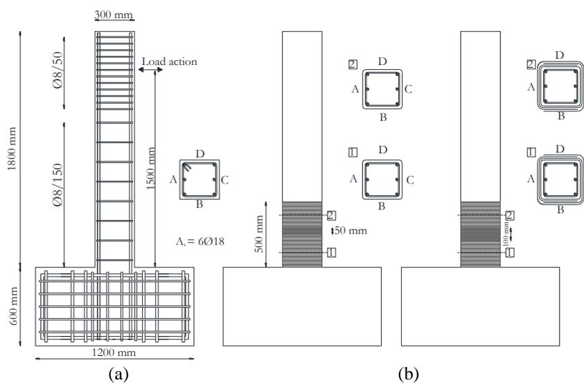
Figure 1. Geometry of specimens: control specimen (a) and confined configurations (b).
