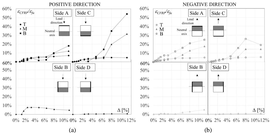
Figure 5. Strain profiles for specimen F1 in positive (a) and negative (b) load direction.
