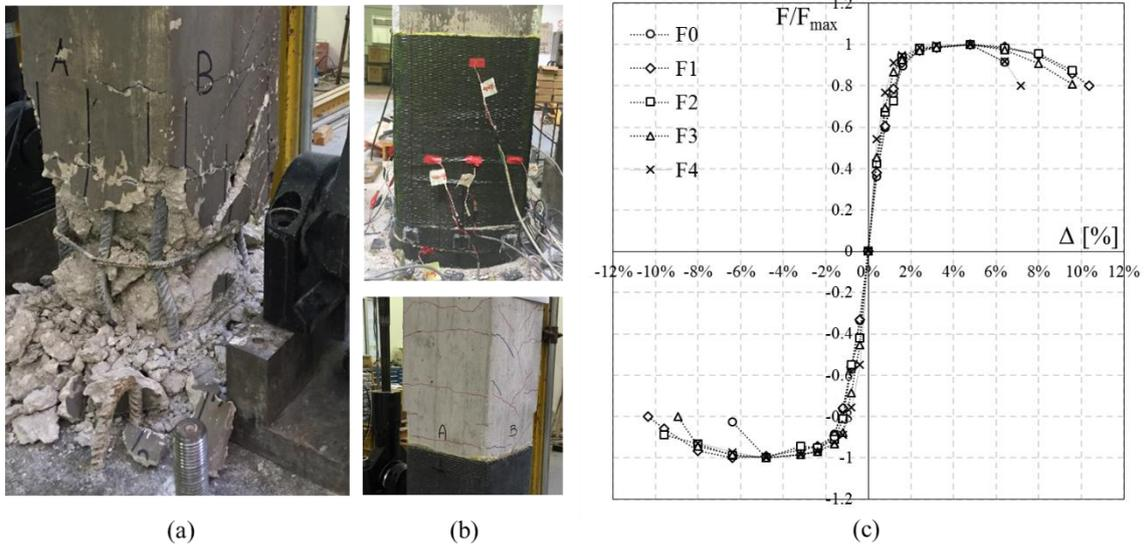
Figure 3. Damage pattern on control specimen (a), on confined specimens (b) and normalized experimental force-drift envelope curves for the five specimens (c).
