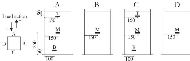
Figure 2. Strain gauges configuration for specimens F1, F2, F3 and F4 (dimensions in mm).
