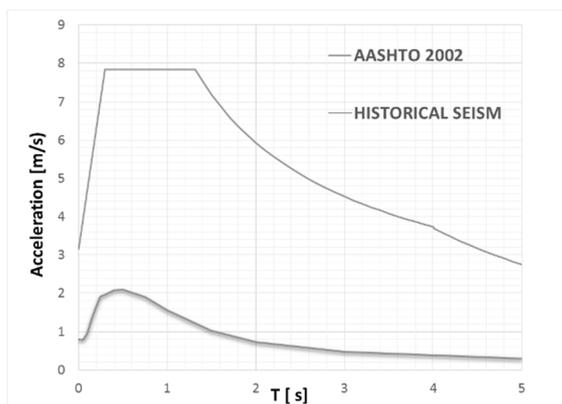
Figure 3. Comparison of AASHTO design spectrum and historic seism spectrum previously experienced by the bridge
