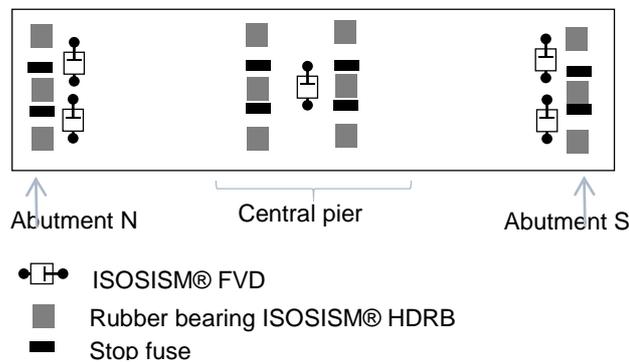
Figure 5. Layout of the bridge for transversal retrofitting
