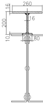
Figure 9. T profile welded on transverse beam
