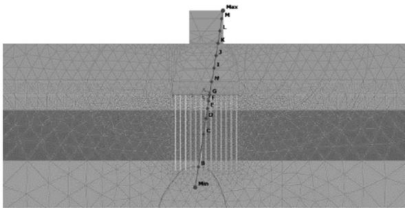
Figure 2. FE model of piers with soil-structure interaction
