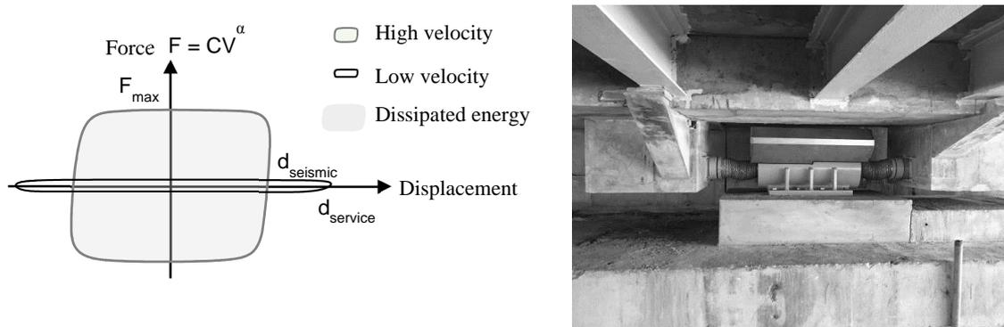
Figure 6. Fluid Viscous Dampers: Behaviour law and picture of FVD installed on pier
