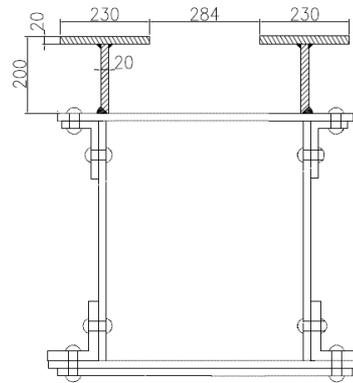
Figure 10. T profiles welded on top chord
