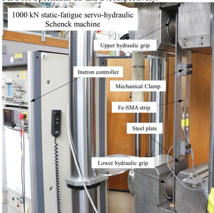
Figure 4. Loading test setup.
