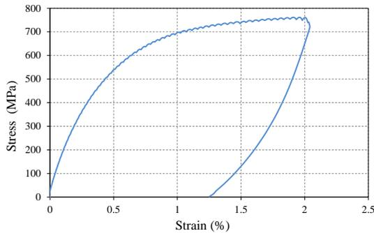
Figure 5. Stress-strain behavior during prestraining of a Fe-SMA strip.
