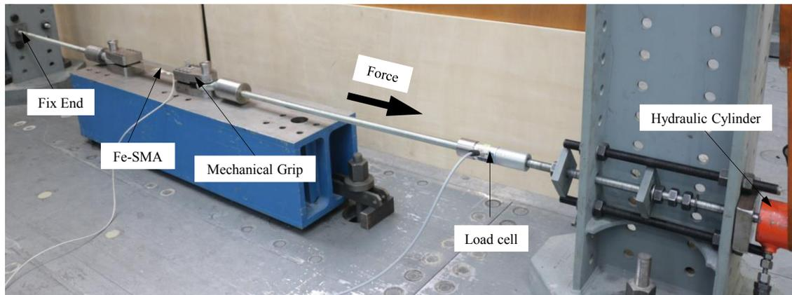
Figure 2. Different elements of the prestraining setup.
