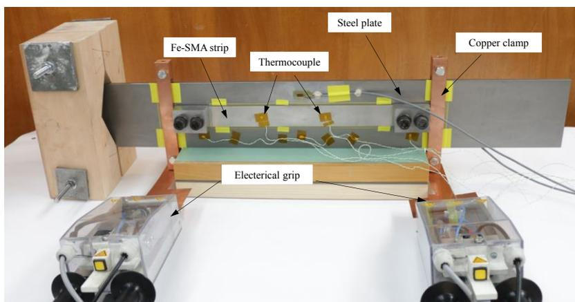
Figure 3. Different elements in the activation setup.
