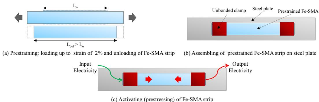
Figure 1. Schematic procedure of steel plate strengthening with Fe-SMA strips.
