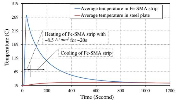
Figure 6. Evolution of temperature in the Fe-SMA strip and the steel plate during activation process for Specimen S3.
