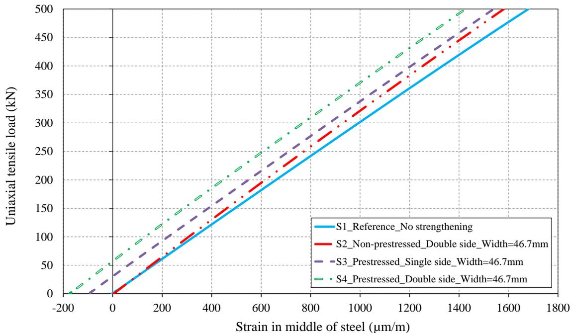
Figure 7. Load-strain behavior of tested specimens subjected to quasi-static tensile loading.
